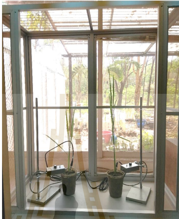
Figure 3.2 AC-DC electropenetrograph recording; rice in plastic pot tray inside the Faraday cage.
