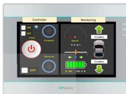
Fig. 10. Dashboard HMI for control systems
