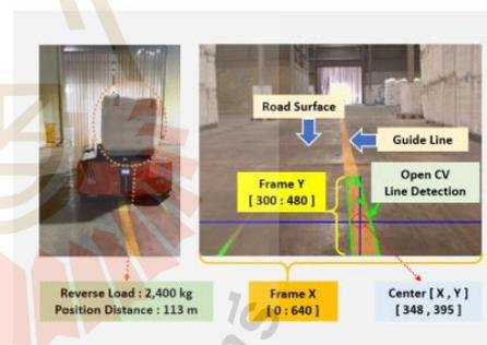
Fig. 17. EV reverse line detection
