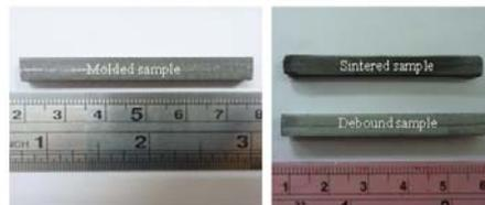
Figure 3. a) Molded sample, b) debound and sintered samples.
