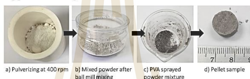
Fig. 3 Warm pellet molding for FP-1 to FP-4 formulas.
