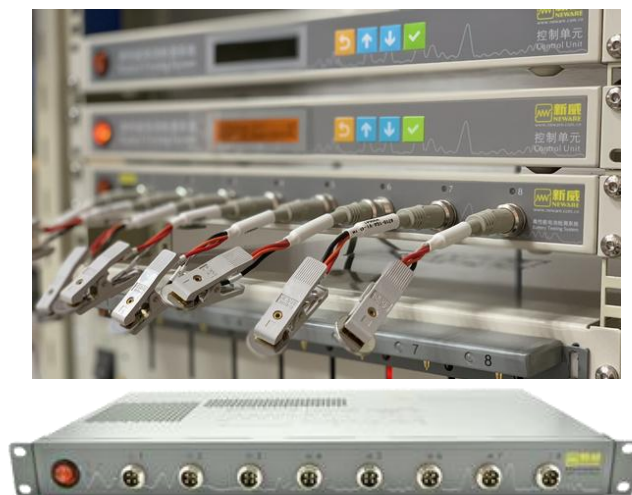
Figure 3.6 Battery Capacity Measurement using Neware BTS4000-5V10mA/5V50mA Systems.
