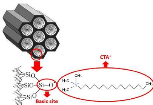
Figure 2.3 An illustration of the MCM-41 structure's basic siloxy site with charge compensation provided by \text{CTA}^+ or CTAB (Zapelini I. W. et al., 2018).
