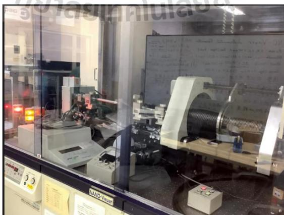
**Figure 3.3** Small-Angle X-ray Scattering (SAXS) instrument at room temperature.
