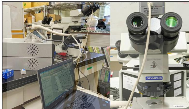
**Figure 3.2** Polarized Optical Microscopy (POM) instrument.
