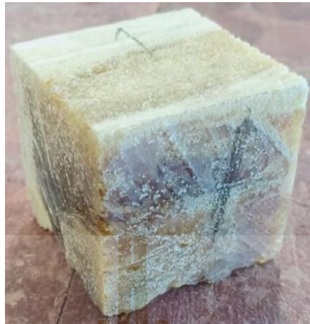
Figure 4.21 PU foam texture of the specimen obtained by injection into the mold.
