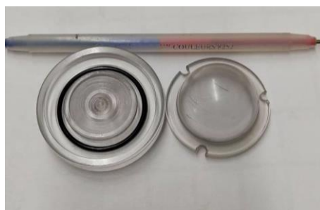
Figure 3.3 An airtight sample holder covered with a PMMA dome.
