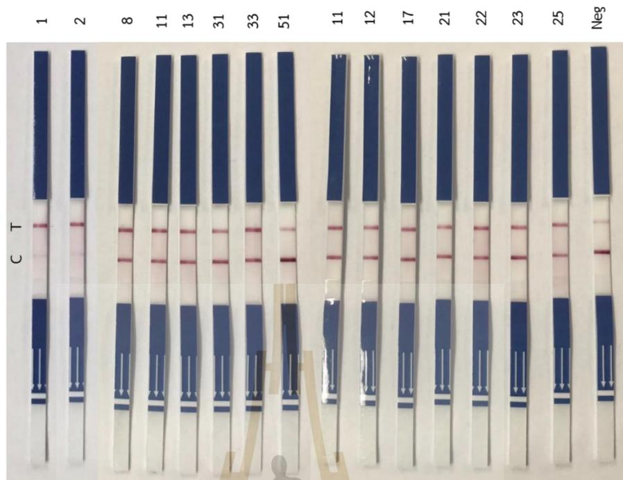
**Figure 4.10** The qualitative analysis results of LFA. The positive samples of COVID-19 were extracted and converted to cDNA, and then were detected by LFA. Numbers at the light are positive samples of COVID-19. “Neg” represents negative control (without DNA template).
