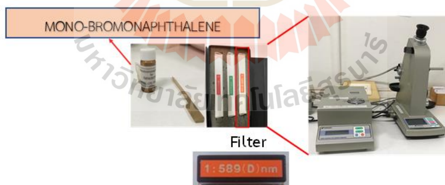
Figure 3.2 A sodium vapor lamp was used as the light source for the Abbe refractometer (ATAGO), which had a wavelength of 589.3 nm (D line), and monobromonaphthalene was used as the contact layer.
