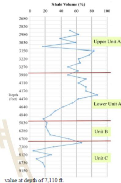
Fig 5. Shale volume of Mae Sod Formation of FA-SS-35-04 well.
