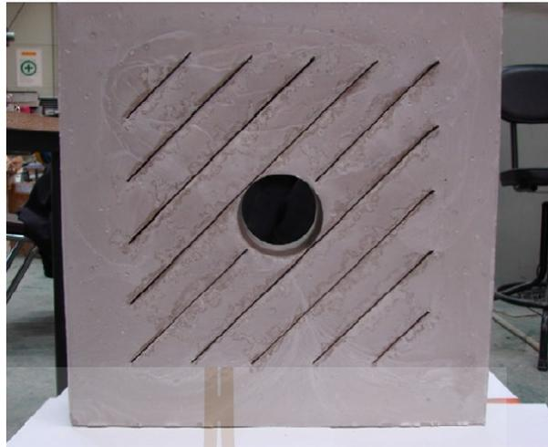
Figure 2.6 Jointed rock model (set dipping at  $30^\circ$ ) (Sagong et al., 2011)
