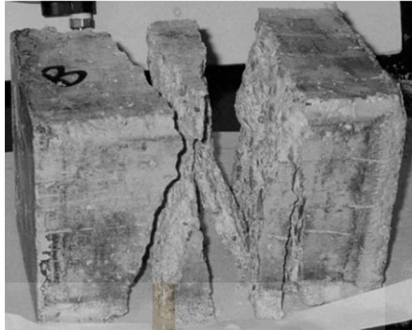
Figure 2.2 Splitting sample under biaxial compression (Sahouryeh et al., 2002)
