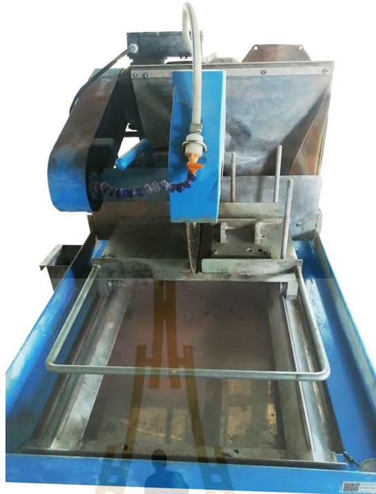
Figure 3.1 High speed saw to cut rock samples
