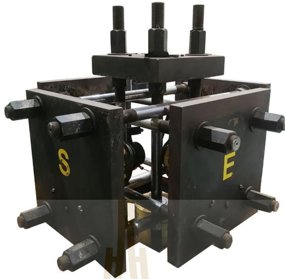
Figure 1.2 True triaxial loading frame (Fuenkajorn et al., 2012)
