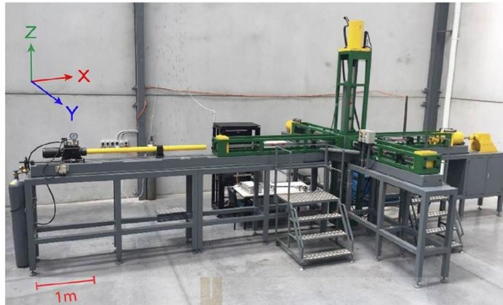
Figure 2.14 Triaxial Hopkinson bar (Liu et al., 2020)
