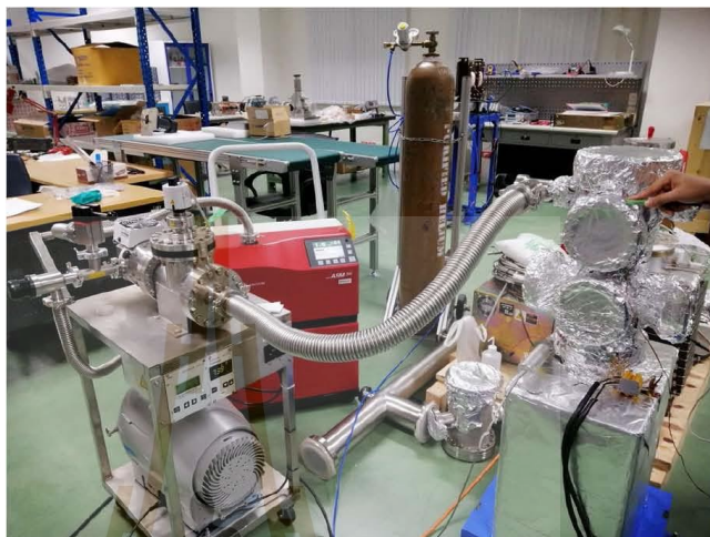
Figure 9. Checking for leaks in the vacuum system.
