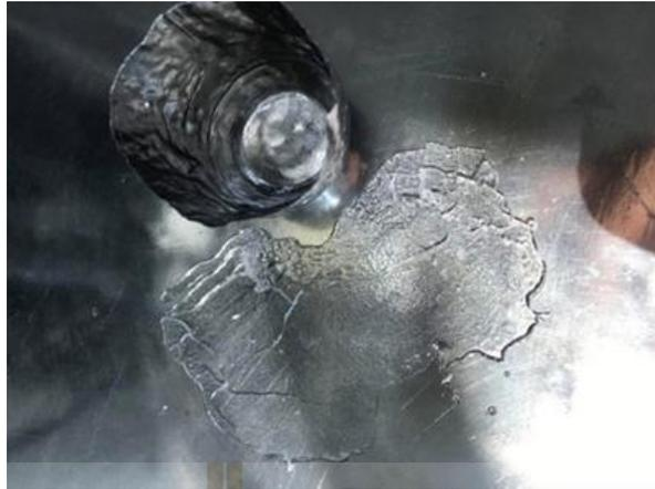
**Figure 4.1** The prepared lithium borate glass by melt-quench technique.
