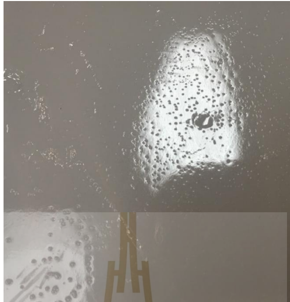
Figure 4.2 Small holes were found on the bottom surface of the gelatin phantom when taken out from the silicone mold with lubricant oil.
