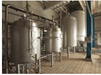
Step 3: fermentation of sugar by bacteria to form lactic acid
