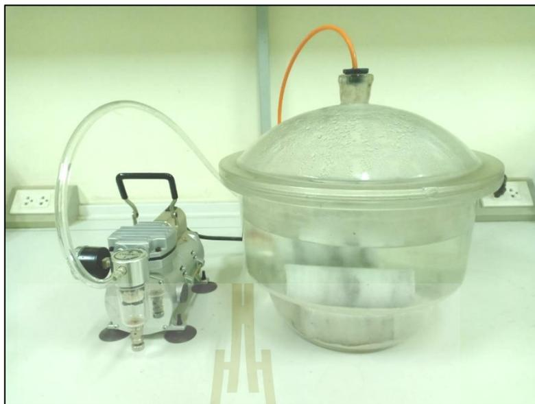
**Figure 4.2** Rock specimens submersed under water in vacuum chamber.
