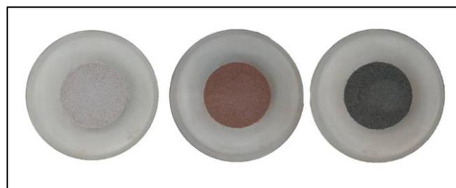
**Figure 3.3** Rock power prepared for XRD analysis.
