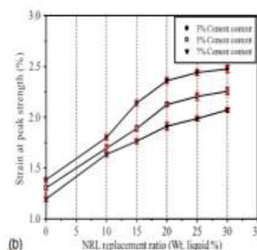
**Fig. 4.** Unconfined compressive test results for different cement contents and NRL replacement ratios: (a) unconfined compressive strength; and (b) strain at peak strength.
