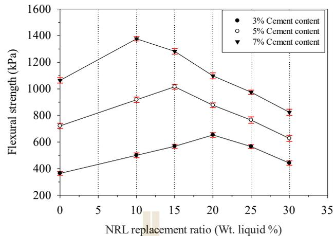
**Figure 3.6** Flexural strength at different cement contents and NRL replacement ratios.
