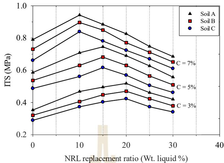
**FIGURE 5.3** Indirect tensile strength for different cement contents and NRL replacement ratios of soil A soil B and soil C.
