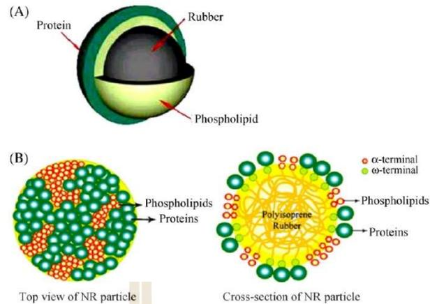
**Figure 2.9** A current model of an NR latex particle surrounded by a double-layer of proteins and phospholipids (Nawamawat et al. 2011).
