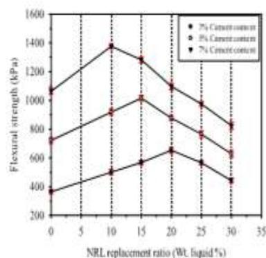
Fig. 6. Flexural strength at different cement contents and NRL replacement ratios.
