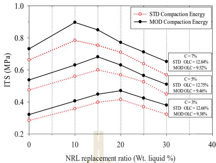
**FIGURE 5.6** Indirect tensile strength for different cement contents and NRL replacement ratios of soil B under STD and MOD compacted energy.
