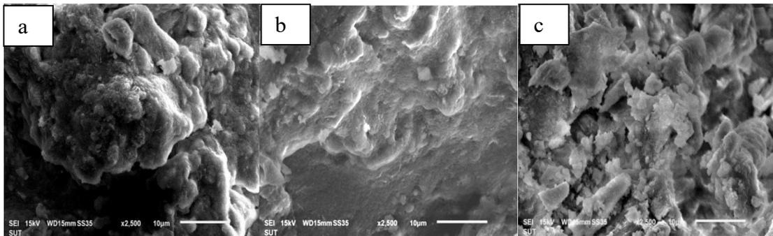
**Figure 3.10** SEM images of samples at (a)3% cement;(b)5% cement and (c) 7% cement and at maximum NRL replacement ratios.
