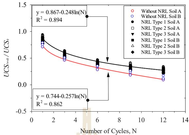
**Figure 4.9** Relationship between  $UCS_{(w-d)}/UCS_0$  and number of w-d cycles at different cement contents and types of NRL for 0% NRL, 10% NRL, 15% NRL, 20% NRL, 25% NRL, and 30% NRL of Soil A and Soil B.
