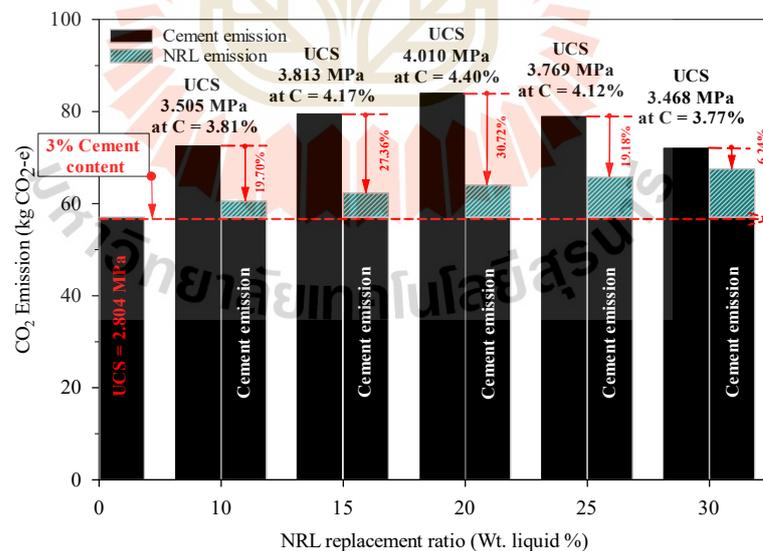
**Figure 4.10** Relationship between CO<sub>2</sub>-e Emission for cement stabilized Soil A and Soil B with and without NRL.
