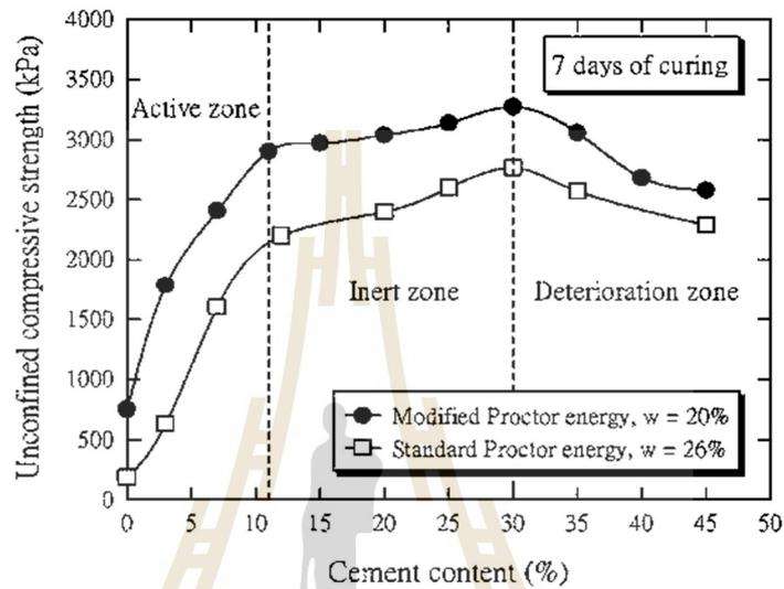
**Figure 2.2** Strength developments as a function of cement content
