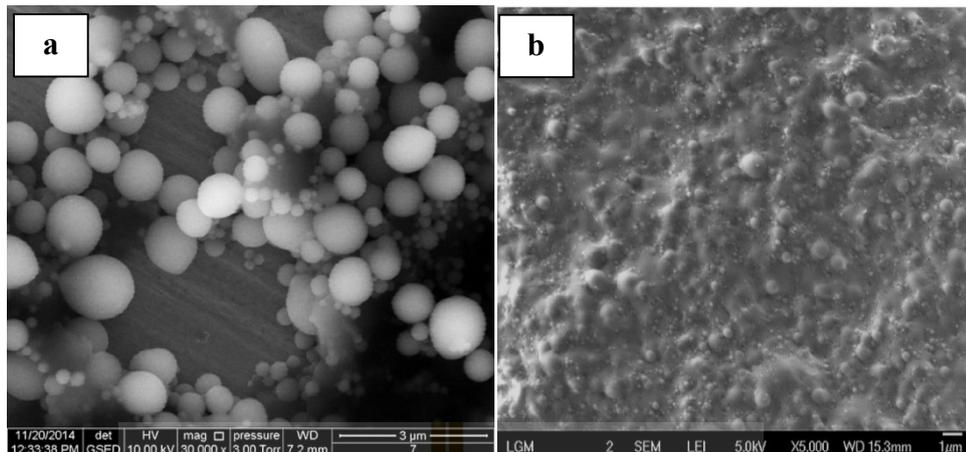
**Figure 2.8** microstructures of particles packing (a) and surface morphology (b) of NRL (Norhanifah et al. 2015)
