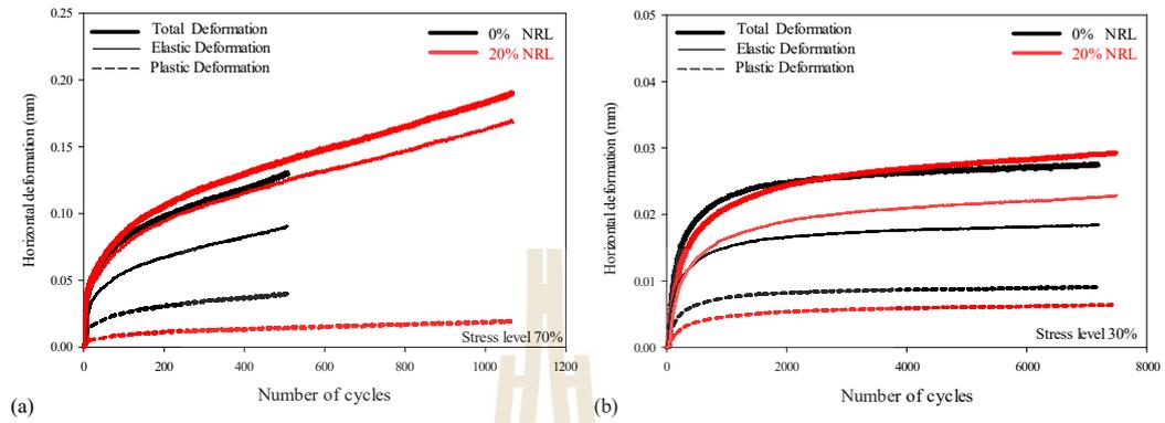
**FIGURE 5.12** Total, elastic, and plastic deformation in zone 1 and zone 2 for cement stabilized Soil A at C=3%, 0%, and 20% NRL replacement ratio at (a) 70% and (b) 30% stress levels.
