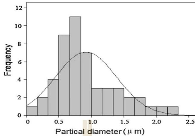
**Figure 2.7** The particle size distribution of uncoalesced NR latex particles dip-coated on a glass substrate imaged one day after preparation (Nawamawat et al. 2011).
