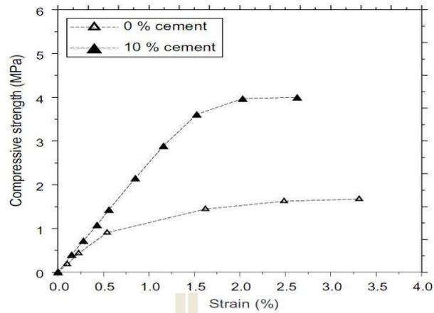
**Figure 2.5** Stress-strain curves for sample under compression (Bahar et al. 2004)
