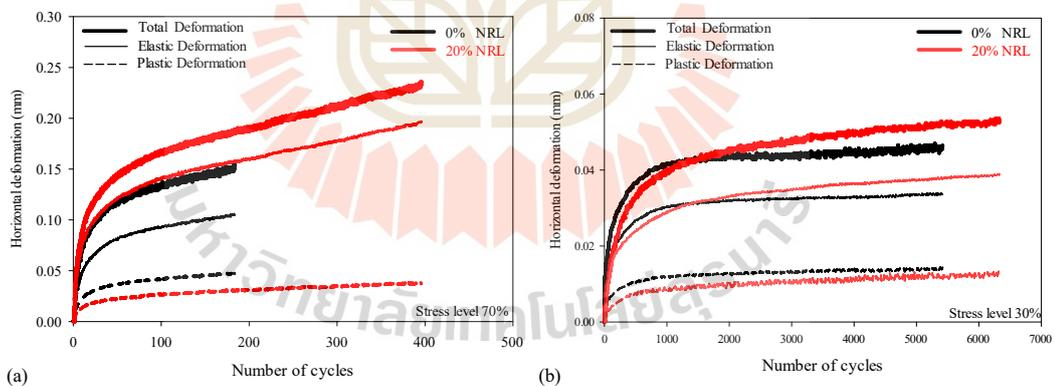
**FIGURE 5.13** Total, elastic, and plastic deformation in zone 1 and zone 2 for cement stabilized Soil at C=3%, 0%, and 20% NRL replacement ratio at (a) 70% and (b) 30% stress levels.
