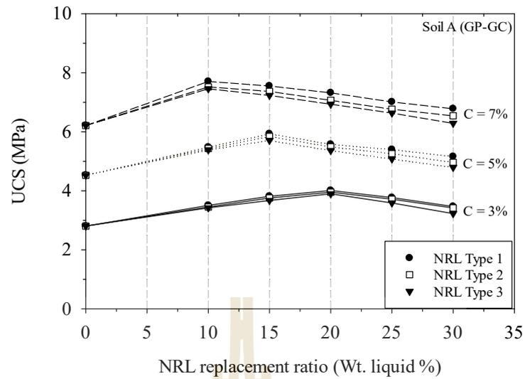
**Figure 4.2** Unconfined compressive strength for different cement contents and NRL replacement ratios of NRL type 1, NRL type 2, and NRL Type 3 of Soil A.
