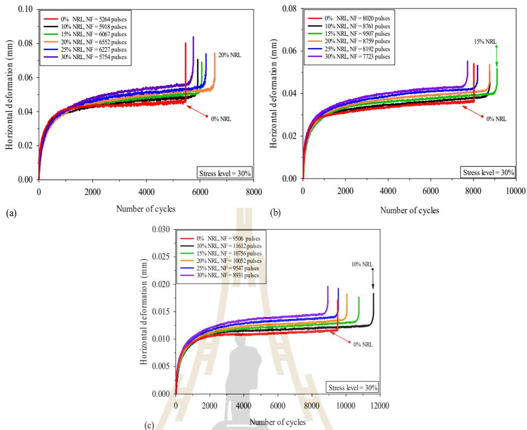
**FIGURE 5.10** Relationship between number of cycles and horizontal deformation of cement stabilized Soil C for (a) C=3%, (b) C=5%, and (c) C=7% at different NRL replacement ratios at 30% stress level.
