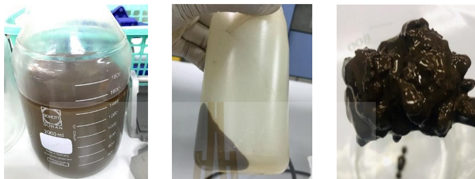
Figure 4.1 Xylan precipitation, xylane centrifugation, wet xylane
