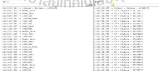
Fig.11.Serial monitor of master controller and Serial monitor of ETT (Model usb to rs485)
