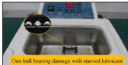
Fig 12 Ball bearing damage in ultrasonic cleaning machine
