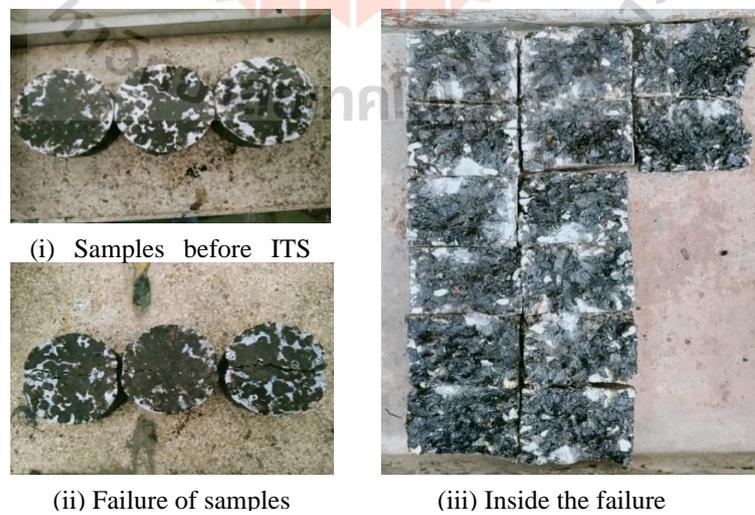
**Figure 3.44** Static ITS test for both un- and conditioned samples
