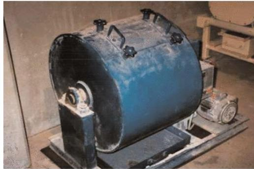
**Figure 2.5** LA abrasion testing machine
