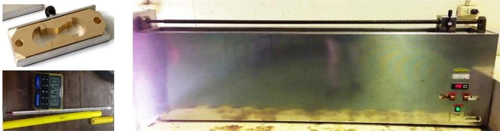
**Figure 3.10** Required apparatus of ductility test
