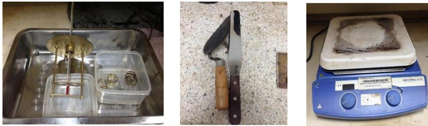
**Figure 3.5** Apparatus of softening point test
