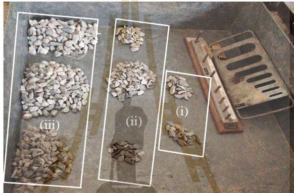
**Figure 3.27** Aggregate separation for flakiness and elongation test
