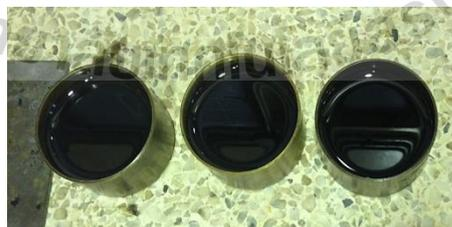
**Figure 3.3** Sample preparation for the penetration test
