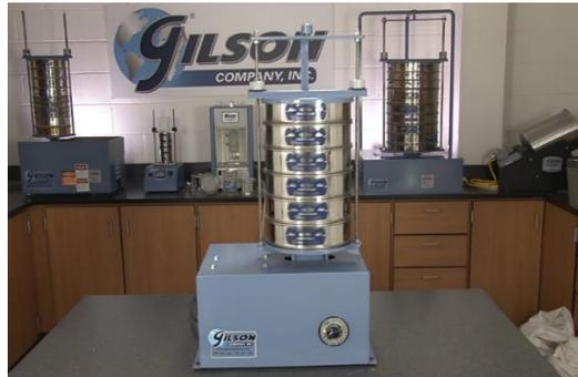
**Figure 2.4** Apparatus of sieve analysis test
