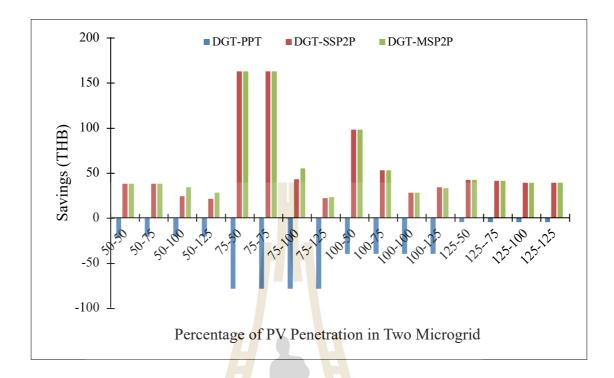
Figure 4.12 Savings in the electricity bill of NG2 in varying PV injection level
