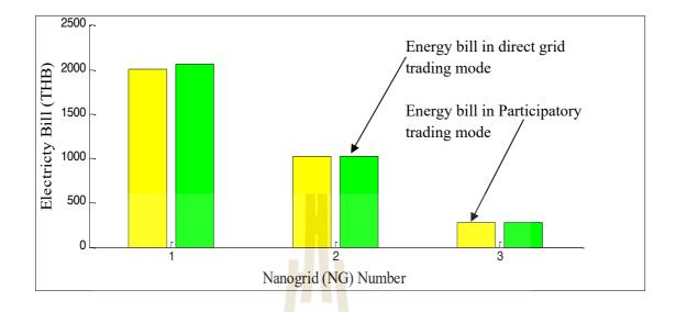
Figure 4.6 Per day electricity bill of NGs of MG2 in PPT and DGT with 100% PV
