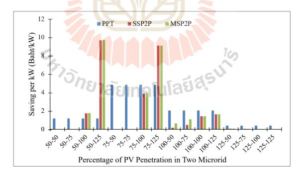
Figure 4.19 Saving per kW PV installation of NG5
