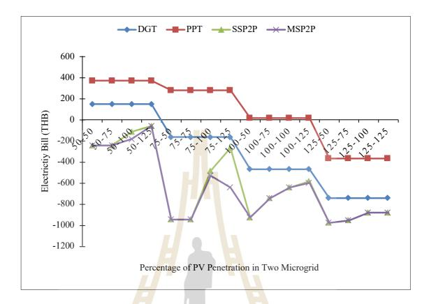
Figure 4.35 Electricity bill of NG2 at varying PV level in interchanged mode
