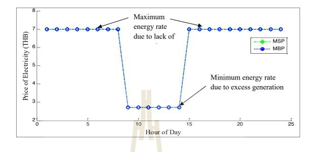
Figure 4.7 MEM Pricing 100% - 100% PV injection case
