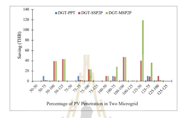
Figure 4.24 Savings in the electricity bill of NG8 in varying PV injection level
