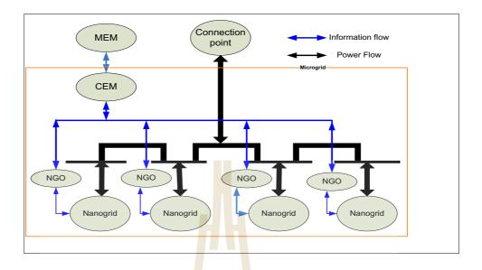
Figure 3.5 Community microgrid operating with various nanogrid
