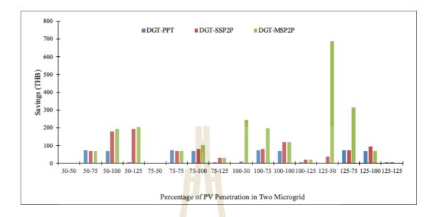
Figure 27 Savings in the electricity bill of MG2 in varying PV injection level
