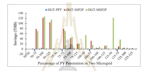
Figure 4.22 Savings in the electricity bill of NG7 in varying PV injection level
