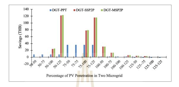
Figure 4.16 Savings in the electricity bill of NG4 in varying PV injection level
