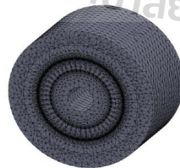
Figure 5. The 3-D mesh of induction motor
