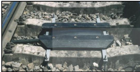
Fig. 5 Radio Frequency (RF) reader for fast moving RFID Tags in high-speed railway application
