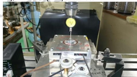
Fig.7 Experimental view to check the axis of the corn holder
