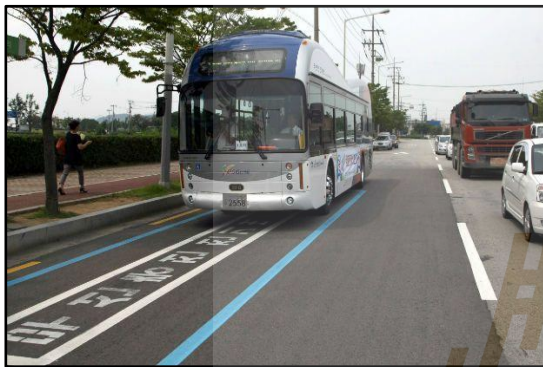
Fig. 2 KAIST OLEV Electric Bus in operation (Installation at bus stops)
