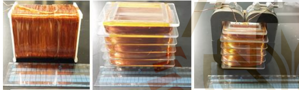
(a) Primary winding (b) Secondary winding (c) Main body Fig.1 Prototype for LF and HV transformer (I)
