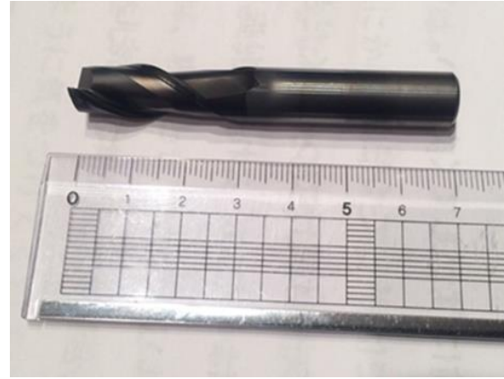
Fig. 3 CVD-diamond coated end-milling tools with the film thickness of 15 \mu\text{m}
