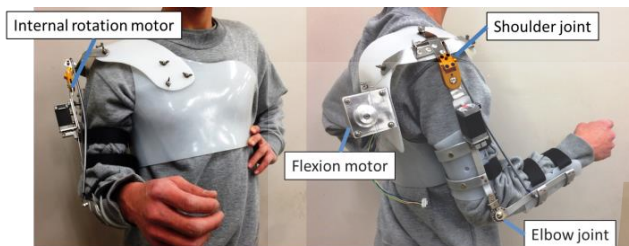
Fig.11: The orthosis manufactured by prosthesist.
