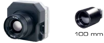
Figure 5: The FLIR Tau 2 thermal camera and its 100mm len used in the experiments
