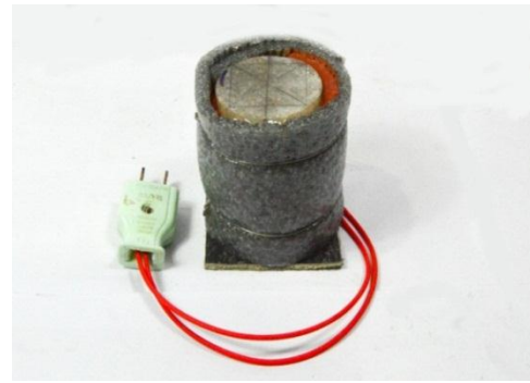
Fig. 2 Salt specimens wrapped with heating tape for elevated temperature testing.
