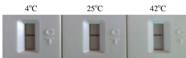
Fig. 9 The drying of the membrane at different temperature for immobilizing antibody.
