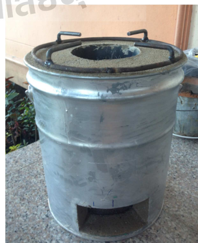
Fig. 2 Low cost small biomass brazier
