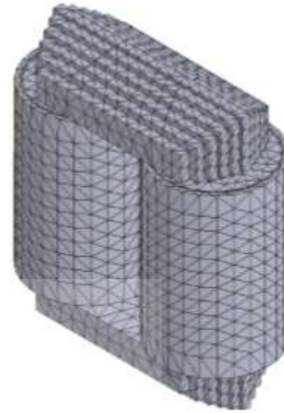
Fig. 5. Tetrahedral elements of the autotransformer
