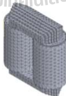
Fig.5. Tetrahedral elements of the autotransformer
