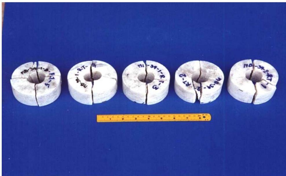
**Figure 3.36** The Saraburi marble specimens failed by ring tension test along the loading diameter.
