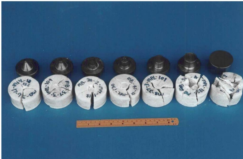
**Figure 3.12** The 67.4 mm-diameter Saraburi marble specimens failed by modified point load tests using various sizes of the loading diameter.
