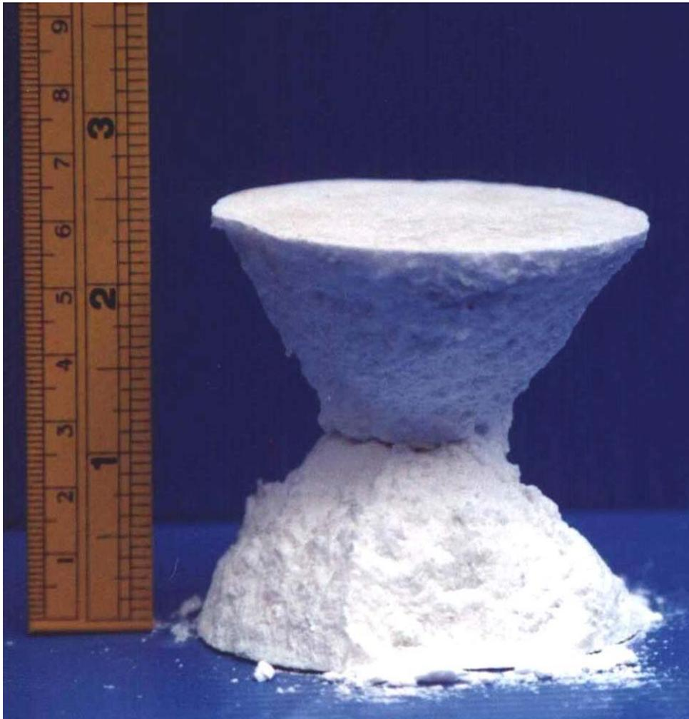
**Figure 3.22** Specimen of Saraburi marble failed under the compressive shear failure mode (conical shape) by uniaxial compressive strength test. ( $D = 67.5$  mm and  $L/D = 1.0$ )
