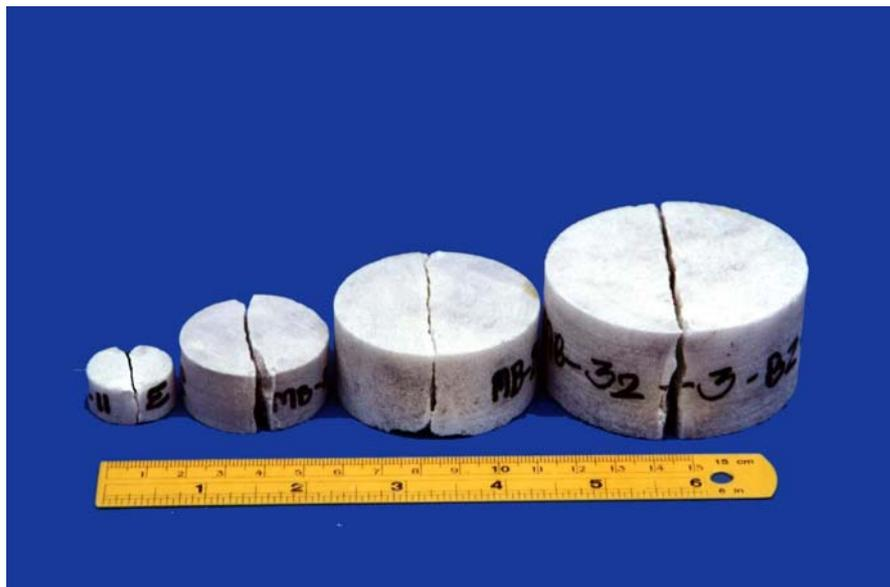
**Figure 3.26** The 22.5, 38.5, 54.0, and 67.4 mm diameter specimens of Saraburi marble failed along the loading diameter in the Brazilian tests.
