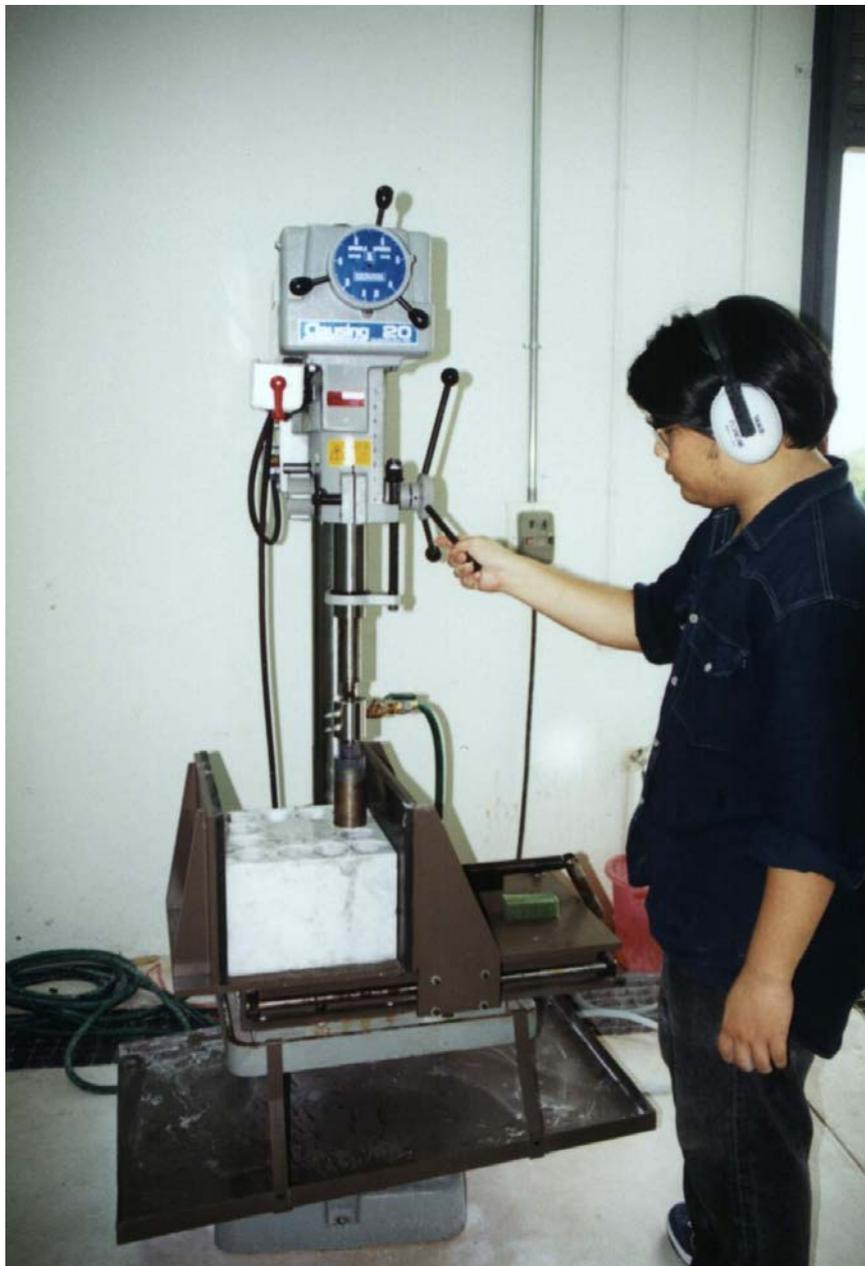
**Figure 3.3** Laboratory core drilling. The core drilling machine (model SBEL 1150) is used to drill core specimens using diamond impregnated bit with diameters varying from 22.5 to 92.5 cm.
