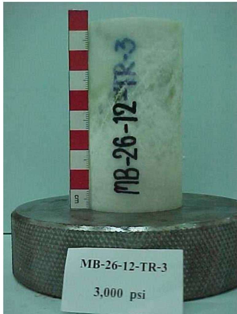
**Figure 3.28** A 54 mm diameter specimen of Saraburi marble with  $L/D = 2.0$  failed by triaxial compressive strength test at confining pressure ( $\sigma_3$ ) 20.7 MPa (Sample No. MB-26-12-TR-3).
