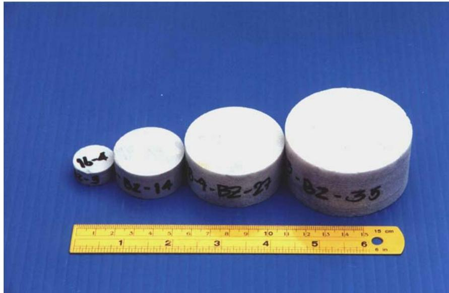
**Figure 3.24** Saraburi marble specimens with diameters varying from 22.5, 38.5, 54.0, to 67.4 mm with  $L/D = 2.5$  for Brazilian tensile strength tests.
