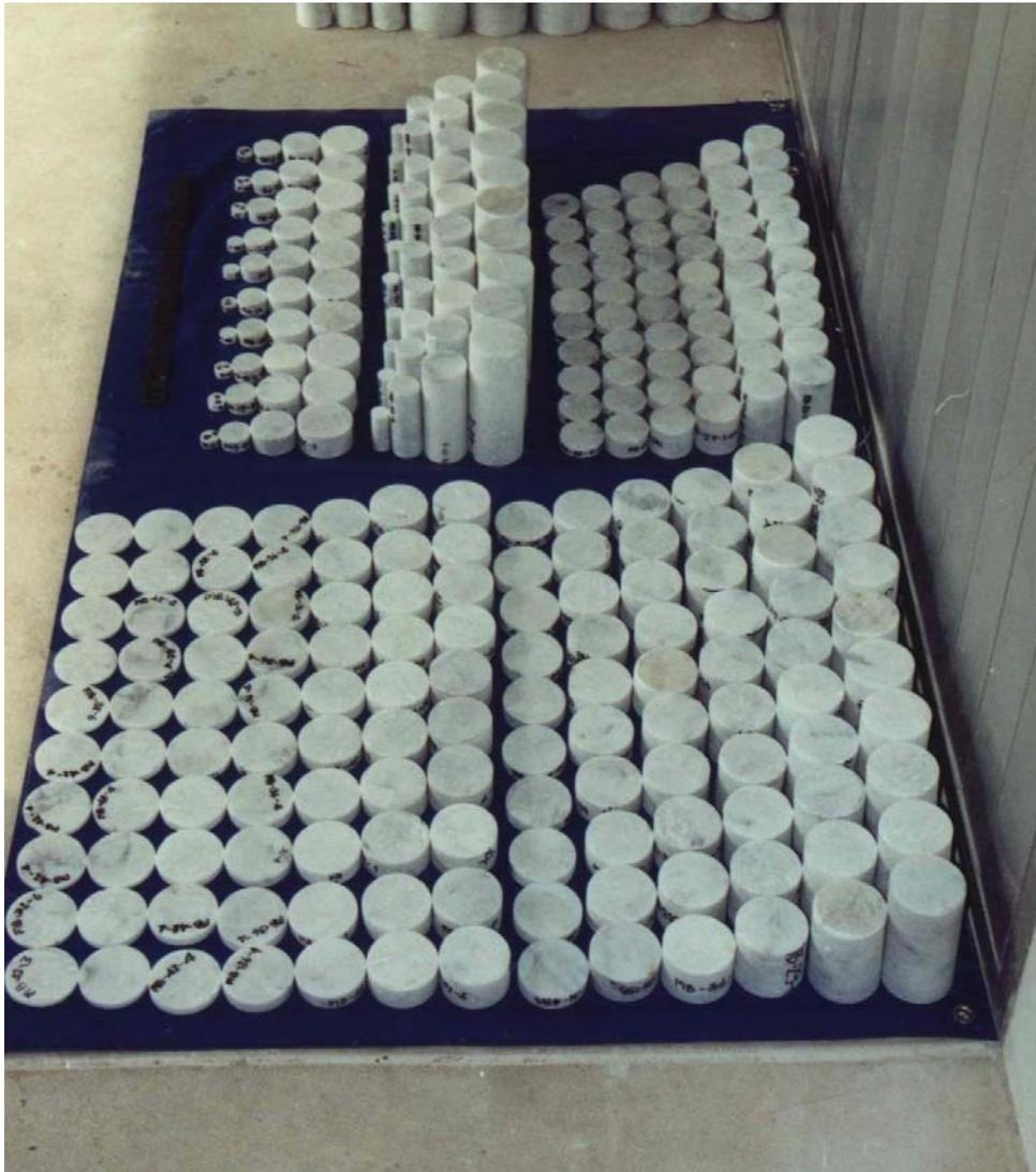
**Figure 3.7** Some Saraburi marble specimens prepared for testing with various sizes and shapes.
