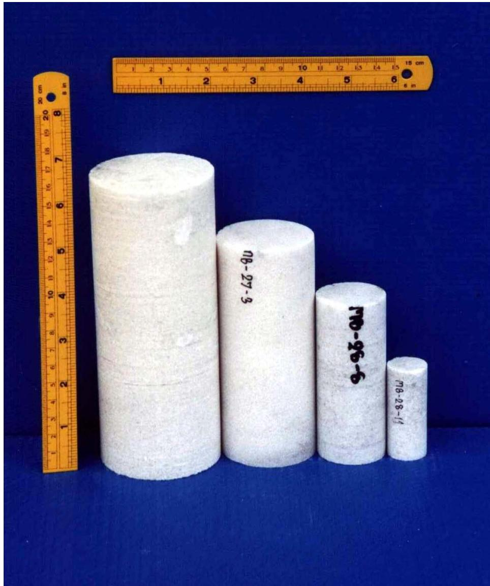
**Figure 3.17** Saraburi marble specimens with diameters varying from 22.5, 38.5, 54.0, to 67.4 mm. They are prepared for uniaxial compressive strength tests.
