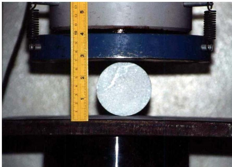
**Figure 3.25** Brazilian test on 67.4 mm diameter specimen of Saraburi marble. The specimen is loaded along the diameter in ELE-ADR2000 compression machine.
