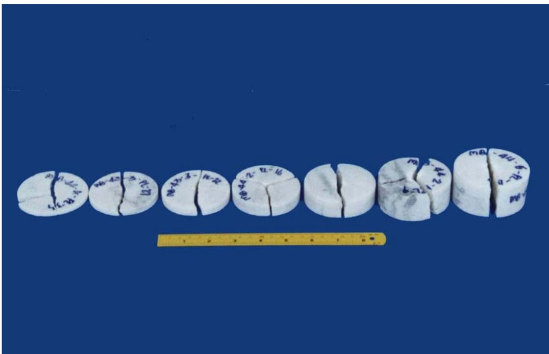
**Figure 3.32** The 67.4 mm diameter specimens of Saraburi marble failed by the conventional point load tests.
