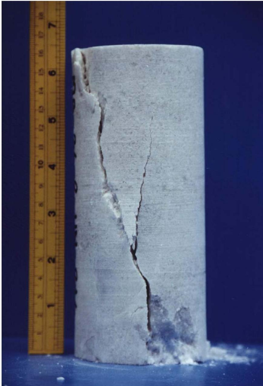
**Figure 3.21** Specimen of Saraburi marble failed under the shear failure mode by uniaxial compressive strength test. The shear failure plane is about 30 degrees from specimen axis. ( $D = 67.5$  mm and  $L/D = 2.5$ )
