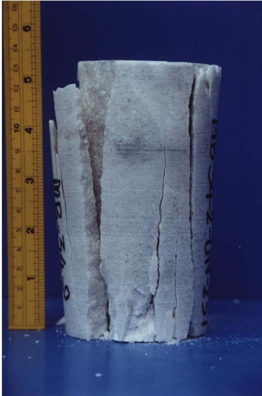
**Figure 3.20** The extension fractures occurs along core specimen axis by uniaxial compressive strength test. ( $D = 67.5$  mm and  $L/D = 2.0$ )
