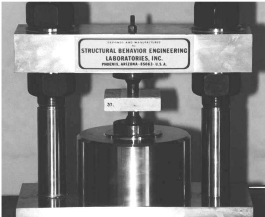
**Figure 3.11** A square disk specimen is tested by the modified point load using 10 mm diameter loading platen.
