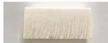
Figure 4: Shape of kerf
