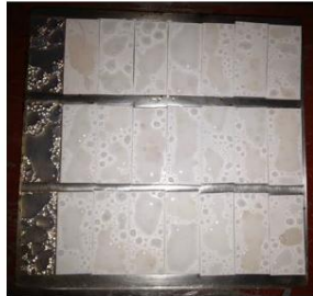
Figure 6: Specimens under vertical corona discharge test.
