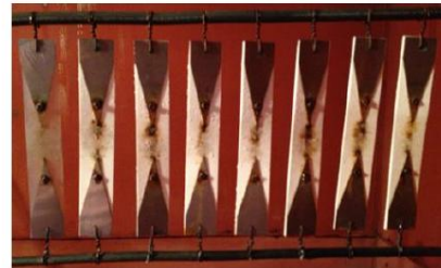
Figure 7: Specimens under parallel corona discharge test.
