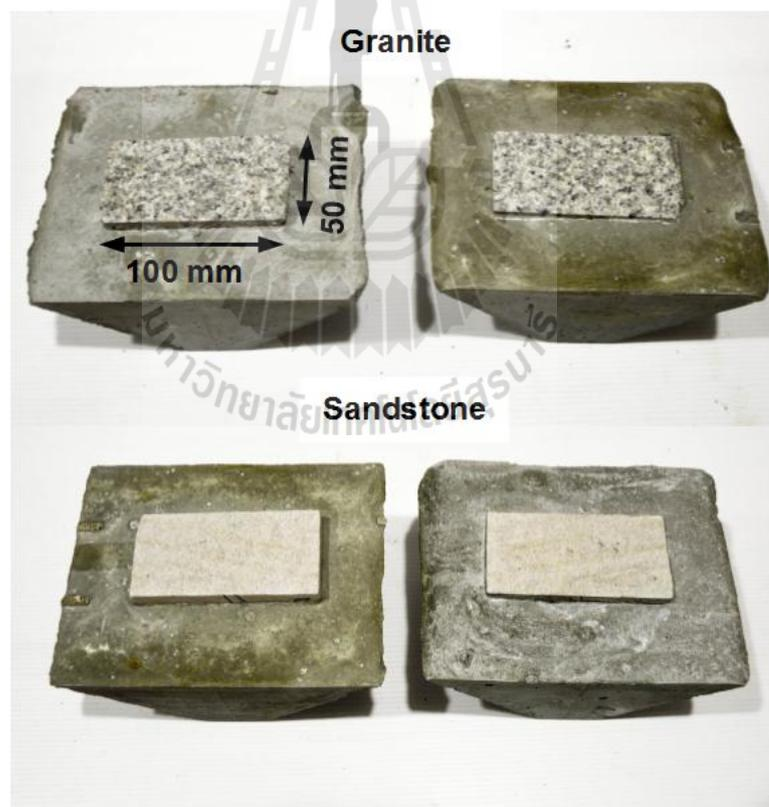
**Figure 3.7** Some specimens prepared for direct shear tests.
