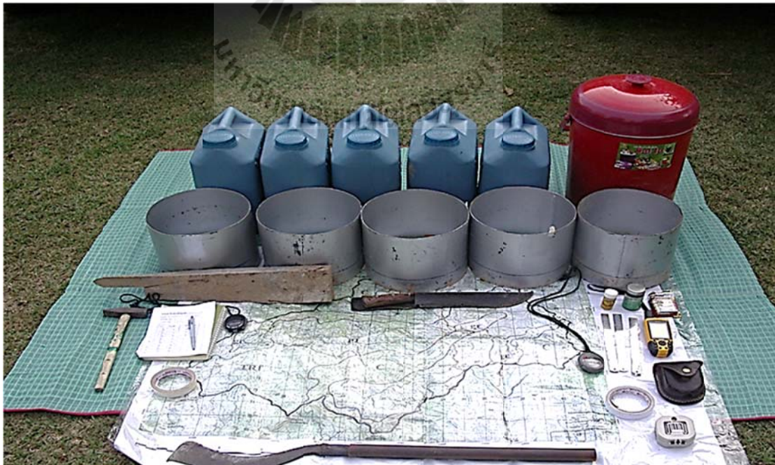
Figure 5.7 The equipment used for infiltration testing.
