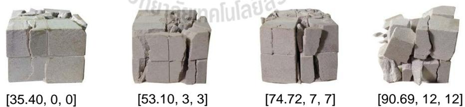
**Figure 5.5** Some post-test specimens of case C. Numbers in brackets indicate  $[\sigma_1, \sigma_3, \sigma_3]$  at failure in MPa.
