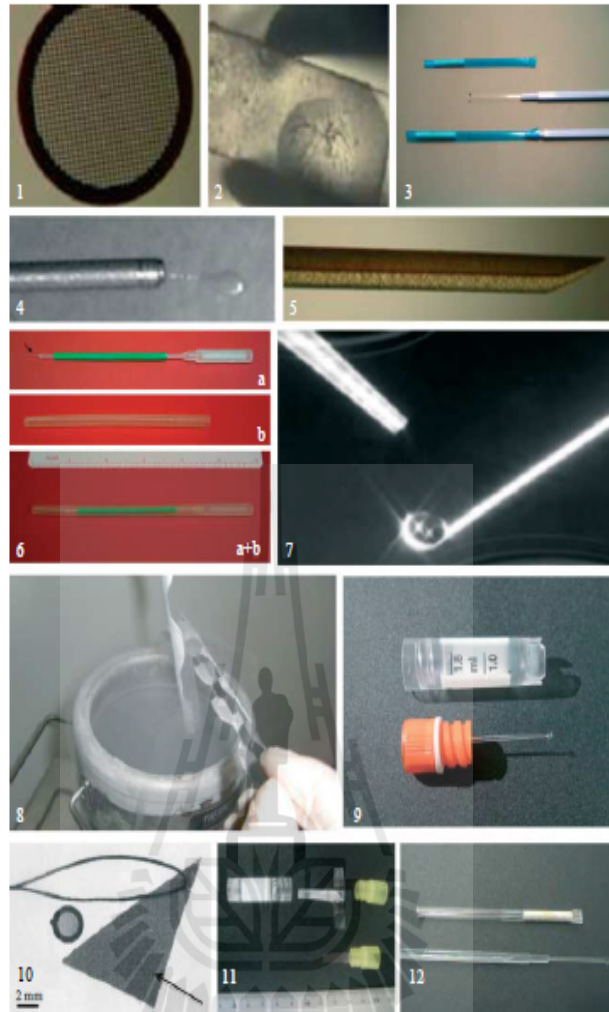
Figure 2.1 Vitrification surface carrier system. (1) electron microscope grid, (2) minimum drop size, (3) Cryotop, (4) Cryoloop, (5) Hemi-straw, (6) Cryoleaf, (7) fiber plug, (8) direct cover vitrification, (9) vitrification spatula, (10) nylon mesh, (12) Vitri-inga. (Source: Saragusty and Arav, 2011).
