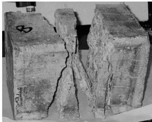
**Figure 2.4** Splitting of concrete sample under biaxial compression (Sahouryeh et al., 2002).
