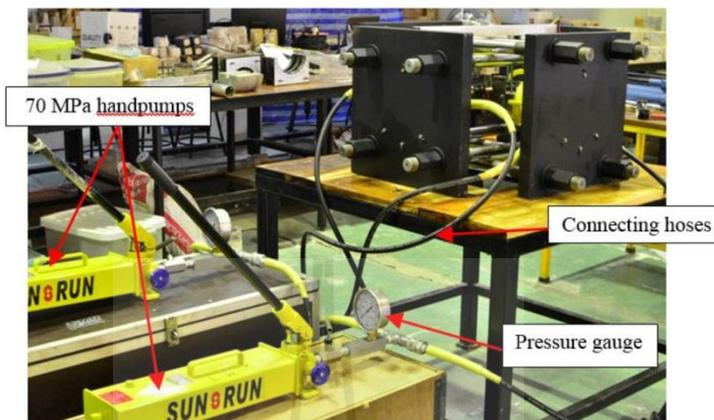
Figure 5. Components of biaxial rock testing devices: main components and accessories.
