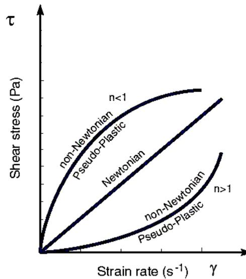
**Figure 2.2** Flow curve of Power law model.
