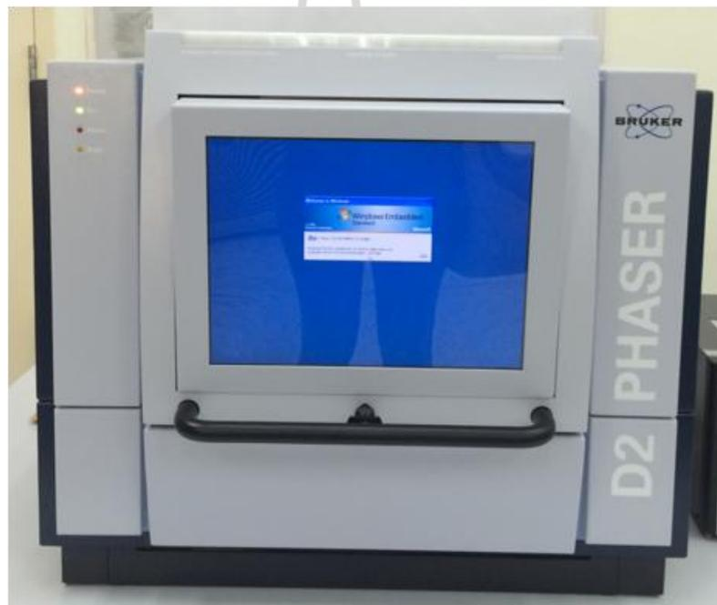
**Figure 3.4** Bruker (D2 Phaser) X-ray diffractometer.
