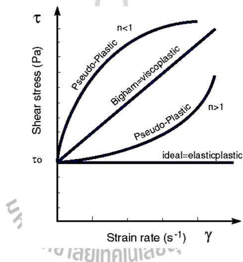
**Figure 2.1** Flow curve for Bingham plastic model.
