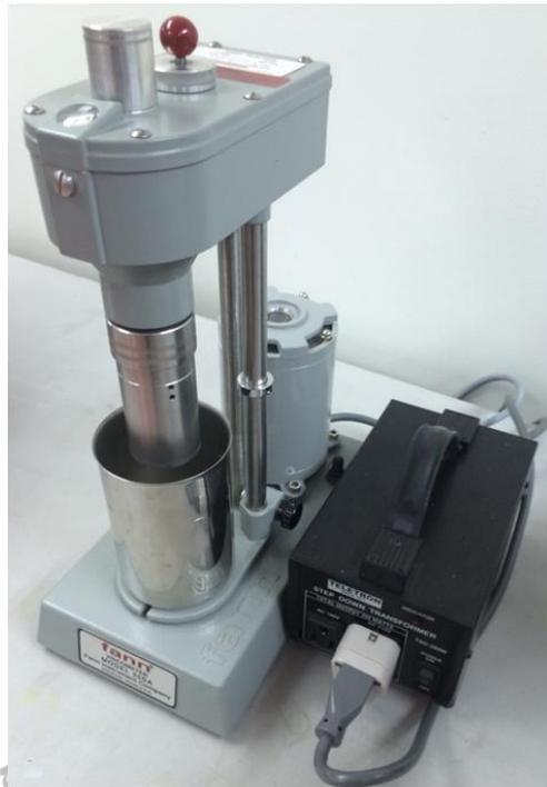
**Figure 3.6** Fann (35SA 115 Volt) Viscometer.
