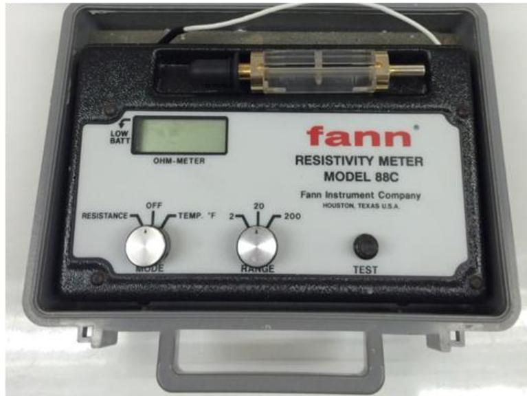
**Figure 3.9** Fann (88C model) resistivity meter.
