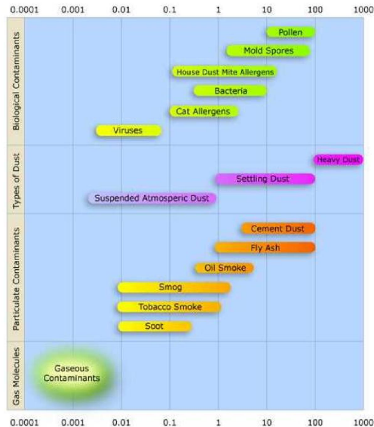
Figure 2.1 Diagram showing size distribution in micrometers ( \mu\text{m} ) of various types of atmospheric particulate matter (PM).
