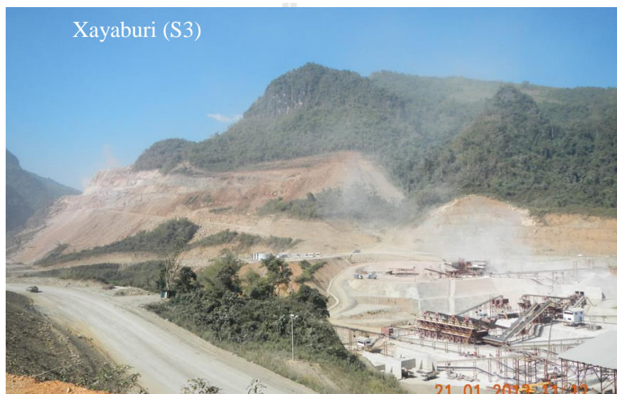
Figure 8 Available limestone quarry and the crushing mill located next to the southwest of dam site.
