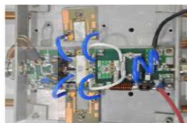
Fig. 17. The prototype of IDPA combined with a negative feedback.
