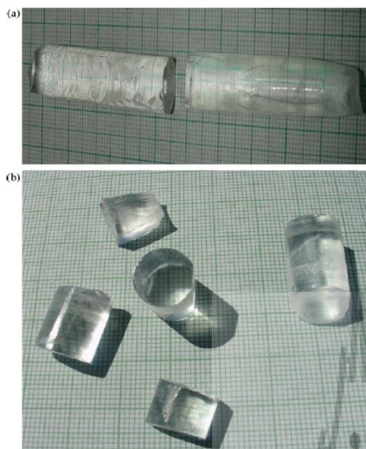
Fig. 1. (a) The KDP crystal with addition of 5 M% KCl grown by SR method. (b) Cut and polished ingot of KDP + 5 M% KCl crystals grown by SR method.
