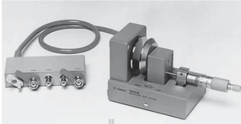
**Figure 3.18** Dielectric test fixture. (Available: <http://www.home.agilent.com/agilent/product.jsp?nid=-34051.536879640.00&cc=TH&lc=eng>).
