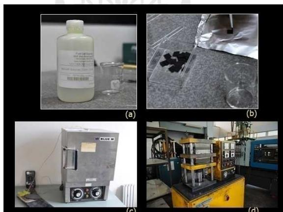
**Figure C.2** Membrane electrode assembly preparations: (a) and (b) To increase the electrochemical reaction at the interface of the membrane and the electrodes, the GDEs have been coated with 5% wt of Nafion solution. (c) The coated GDEs are heated with  $70^\circ\text{C}$  for 1hr. within the oven. (d) The membranes and electrodes are then subjected into the membrane electrode assembly by hot-pressing apparatus.
