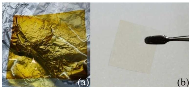
**Figure 4.1** The degraded Nafion membrane before pretreatment (a) and the Nafion membrane after chemical pretreatment (b).
