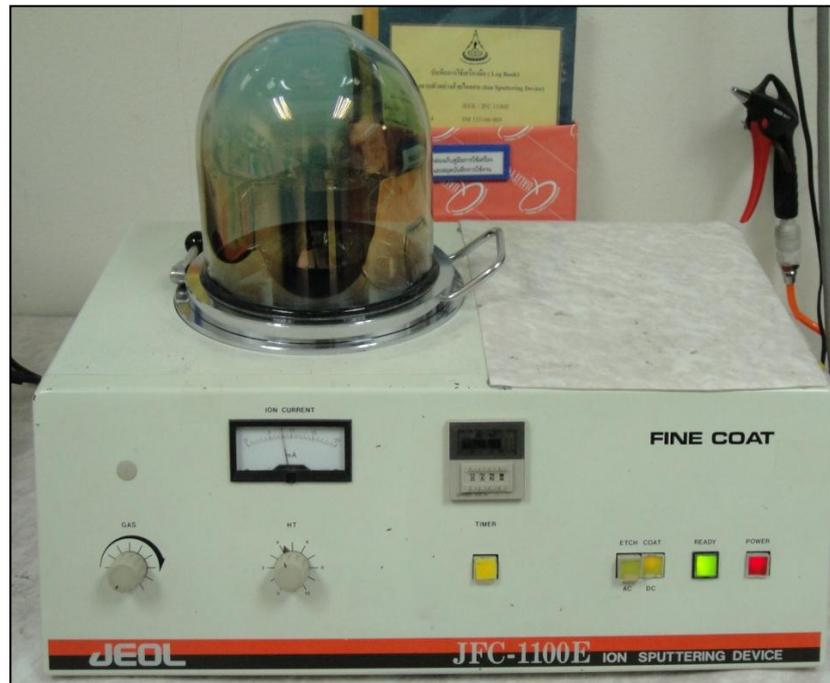
**Figure 3.13** Ion sputtering machine JEOL JCF-1100E.
