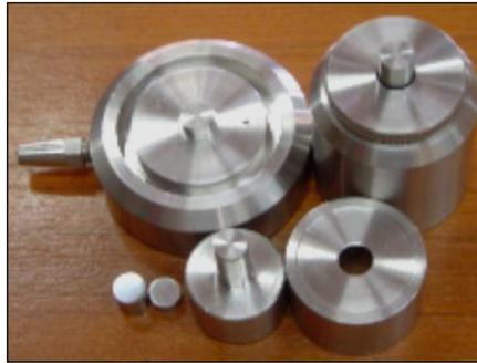
**Figure 3.4** Stainless steel mold for pressing disk samples (diameter = 10 mm).
