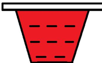
**Figure 3.8** Arrangement of samples in alumina crucible, white is alumina cover plate, red is alumina powder and black are samples.
