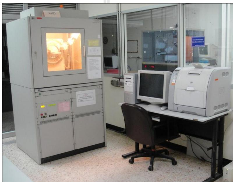
**Figure 3.10** X-ray diffractometer (Bruker D5005).
