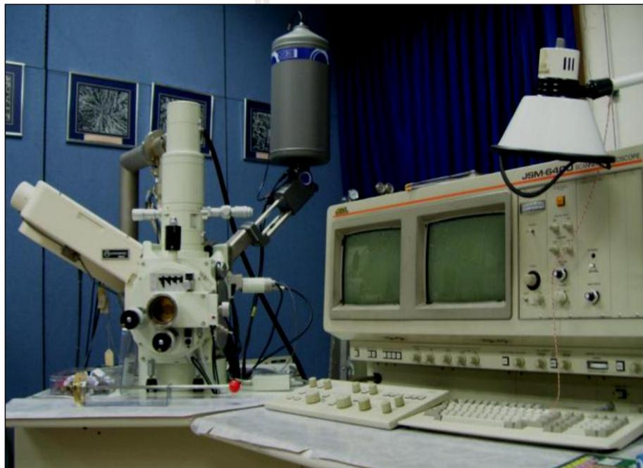
**Figure 3.12** *SEM* instrument, JOEL JSM-6400.
