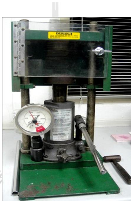
**Figure 3.5** Hydraulic presser CARVER hydraulic unit model #3912.
