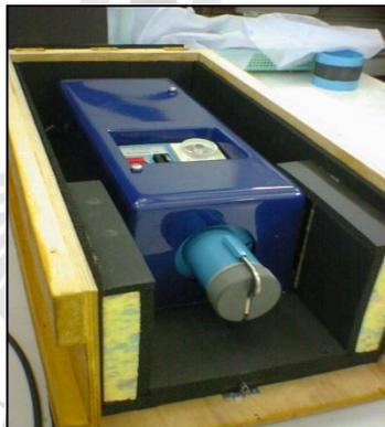
**Figure 3.2** The vibro-milling machine (McCrone micronizing mill).
