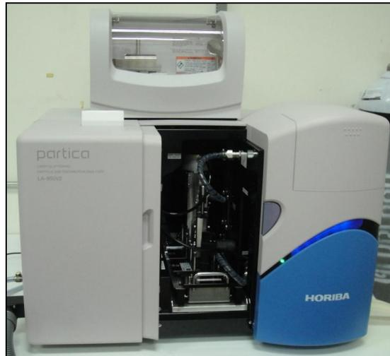
**Figure 3.11** HORIBA Laser Scattering Particle Size Distribution Analyzer LA-950V2.
