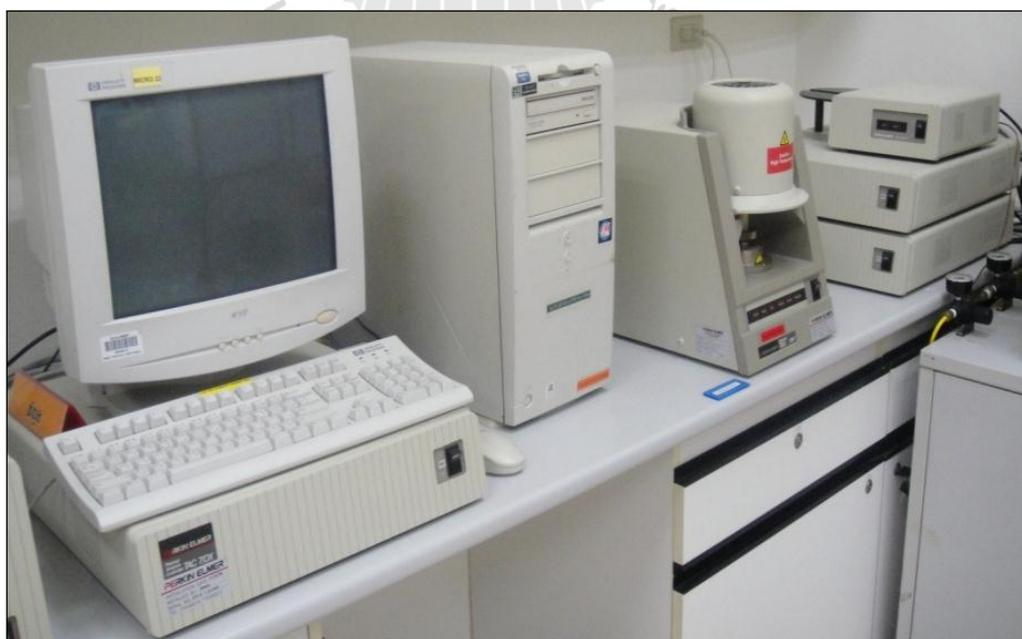
**Figure 3.9** Differential Thermal Analyzer DTA7 instrument by Perkin Elmer.
