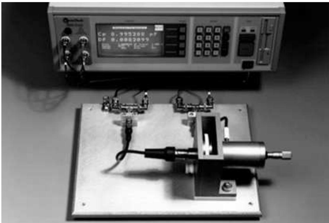
Figure 2.14 LCR meter ([www.tmworld/file/4402](http://www.tmworld/file/4402)).
