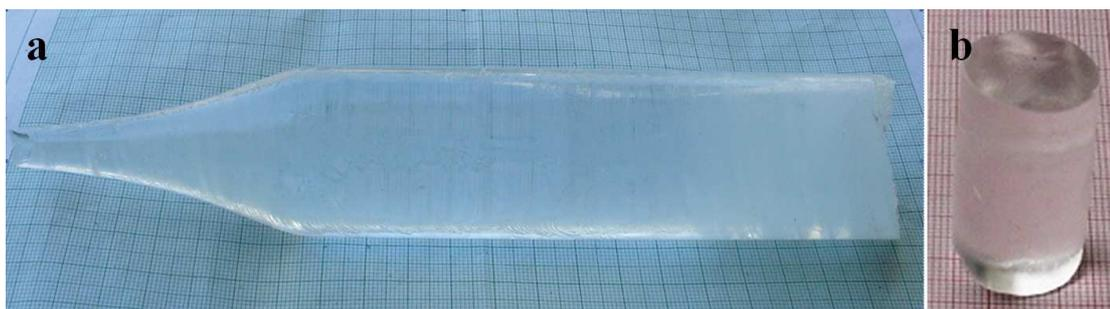
**Figure 3.2** (a) As grown and (b) Cut and polished SR grown Sulphamic acid crystal.
