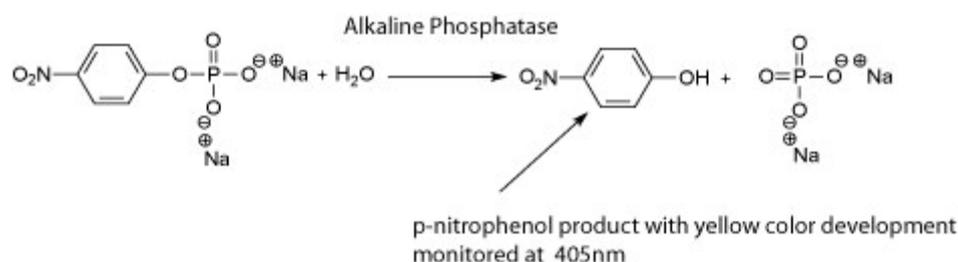
**Figure 66.** Generating p-nitrophenol yellow color product, alkaline phosphatase digest substrate diagram. (From Sigma pNPP data sheet)
