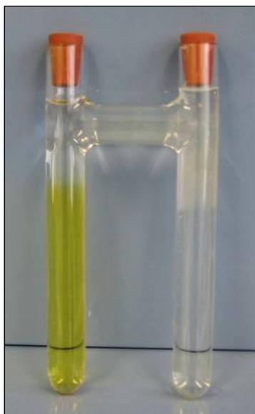
H-tube apparatus with  $[\text{Fe}(\text{L})(\text{CN})_4]^{2-}$  on left
