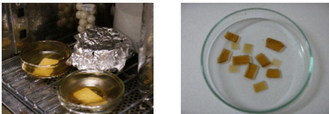
**Figure 3.4** Thin films of ionomers casted from glass disk.
