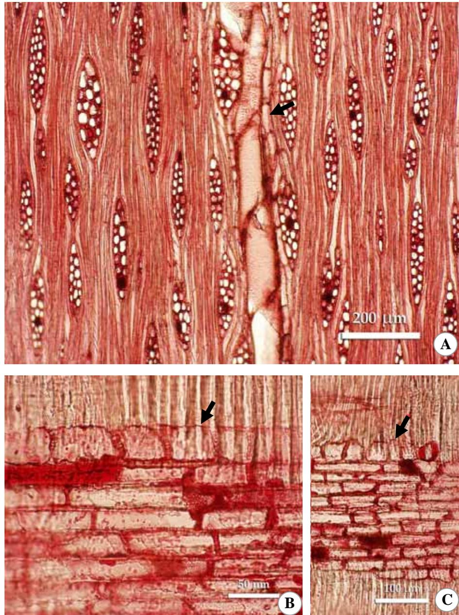
**Figure 4.70** Thin section of *Azadirachta excelsa*. **A.** (Tg) (1 - 2) 3 - 4 seriate non-storied rays, non-septate fibers, and parenchyma strands (arrow). **B.** and **C.** (R) Body ray cells procumbent with 1 row of square/upright marginal cells (arrows).
