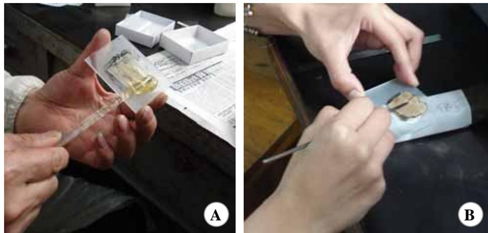
**Figure 3.11 A.** Fixing a specimen with Abienic balsam\* .
