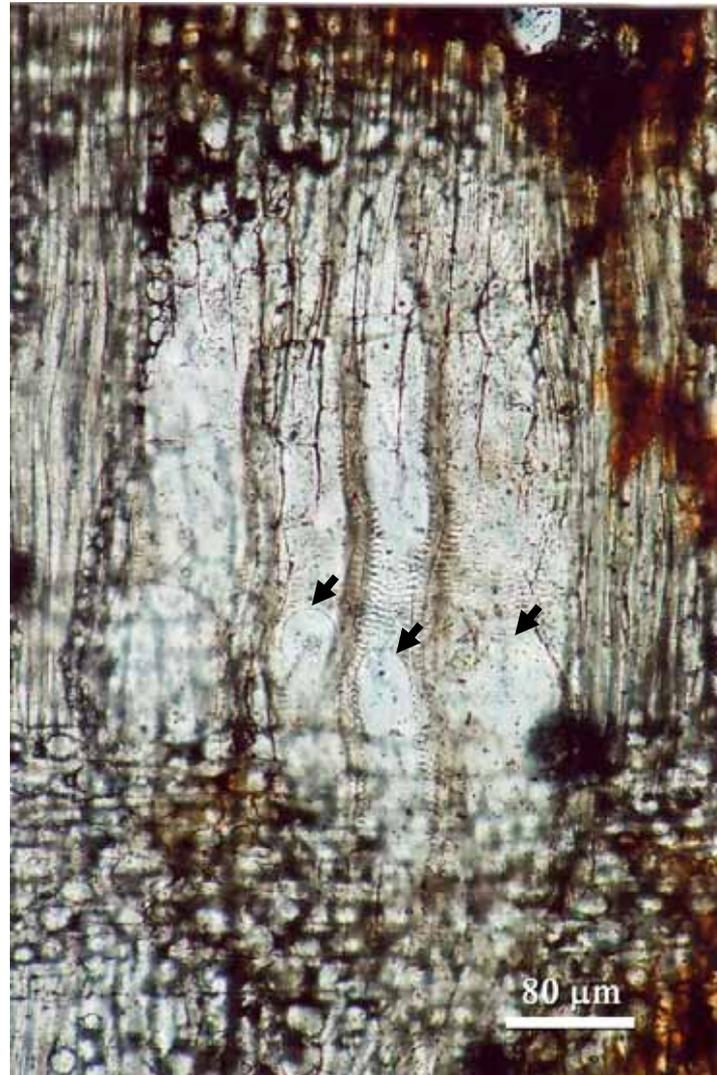
**Figure 4.60** Thin section of O7 in radial section showing simple perforation plates of vessel elements (arrows).
