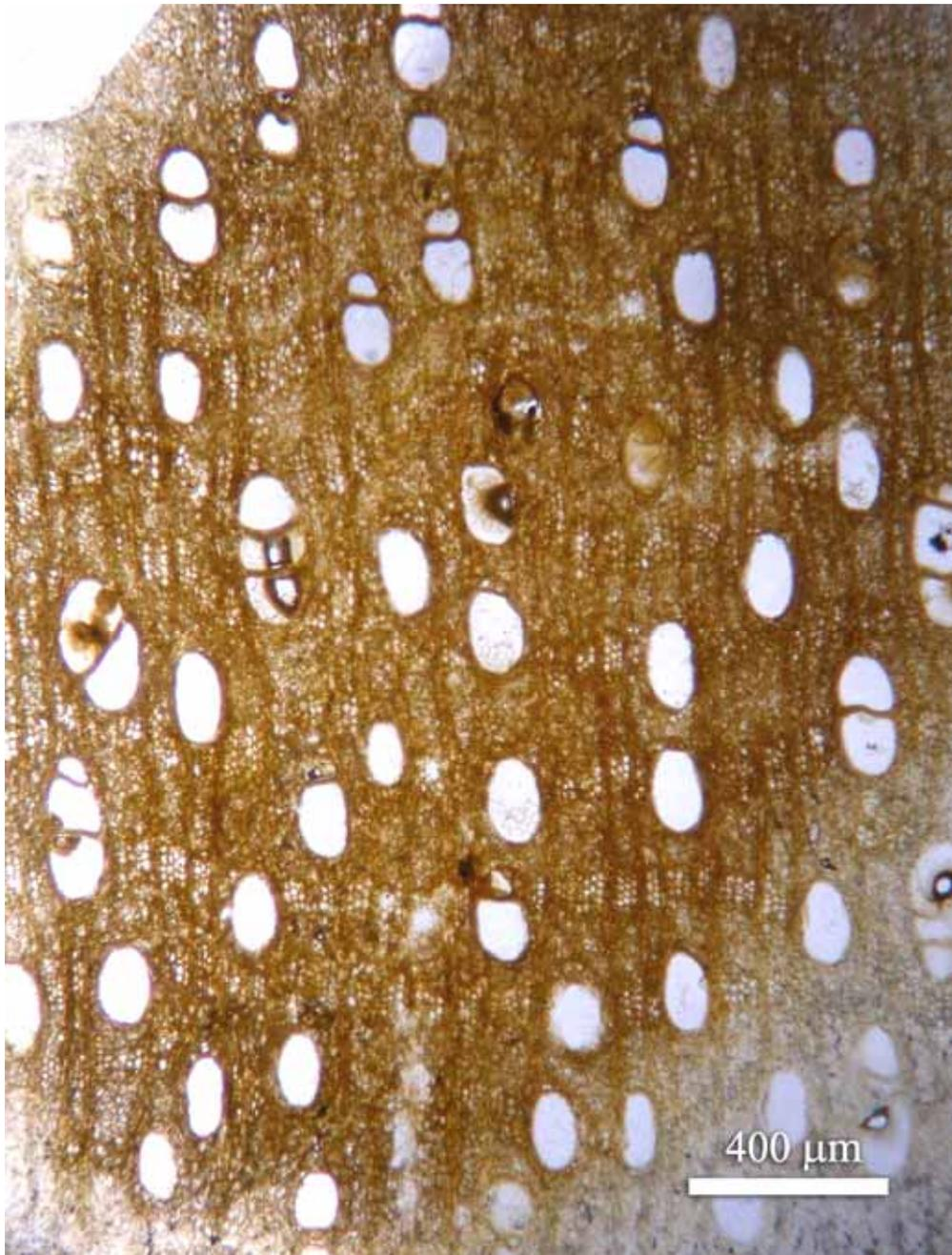
**Figure 4.52** Fossil wood of I2-1 in transverse section showing vessel distribution as diffuse-porous wood. Vessels solitary or some in radial multiples of 2 - 3. Banded parenchyma.
