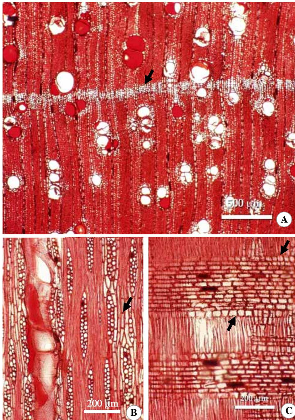
**Figure 4.68** Thin section of *Azadirachta indica*. **A.** (Tv) Solitary vessels common and irregular band of 6 - 10 cells comprising axial parenchyma. **B.** (Tg) Non-storied and (1) 2 - 3 seriate rays. Non-septate fibers and parenchyma strands (arrow). **C.** (R) Body ray cells procumbent with 1 upper and 1 lower row of square/upright marginal cells (arrows).
