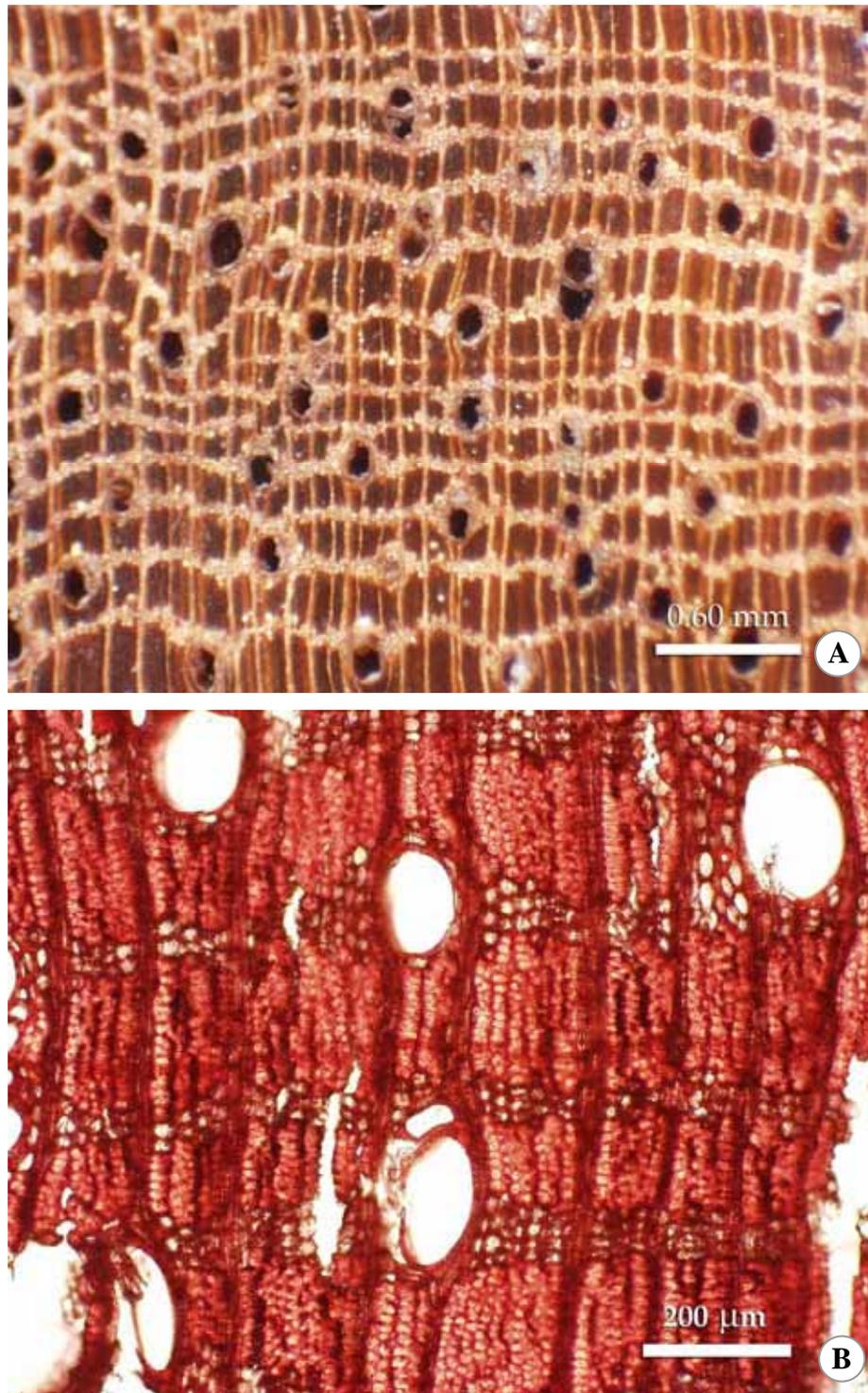
**Figure 4.33** Thin section of modern wood of *Irvingia malayana* in transverse section.
