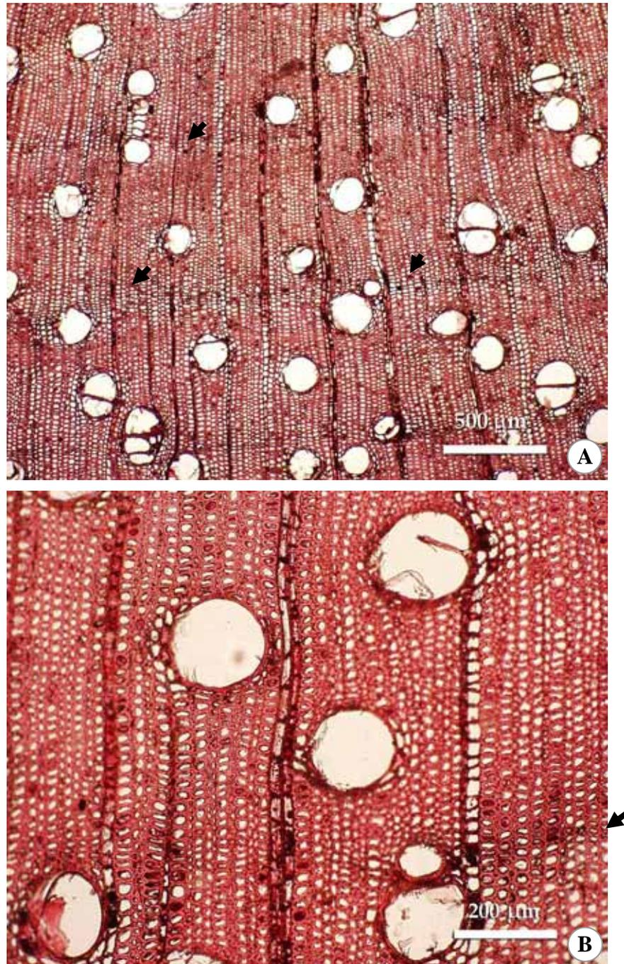
**Figure 4.17** Thin section of *Canarium venosum* in transverse section. **A.** and **B.** Vessels solitary and in radial multiples of 2 - 3 (4), axial parenchyma scanty to vasicentric narrow sheath, parenchyma in marginal or seemingly marginal bands (arrows).
