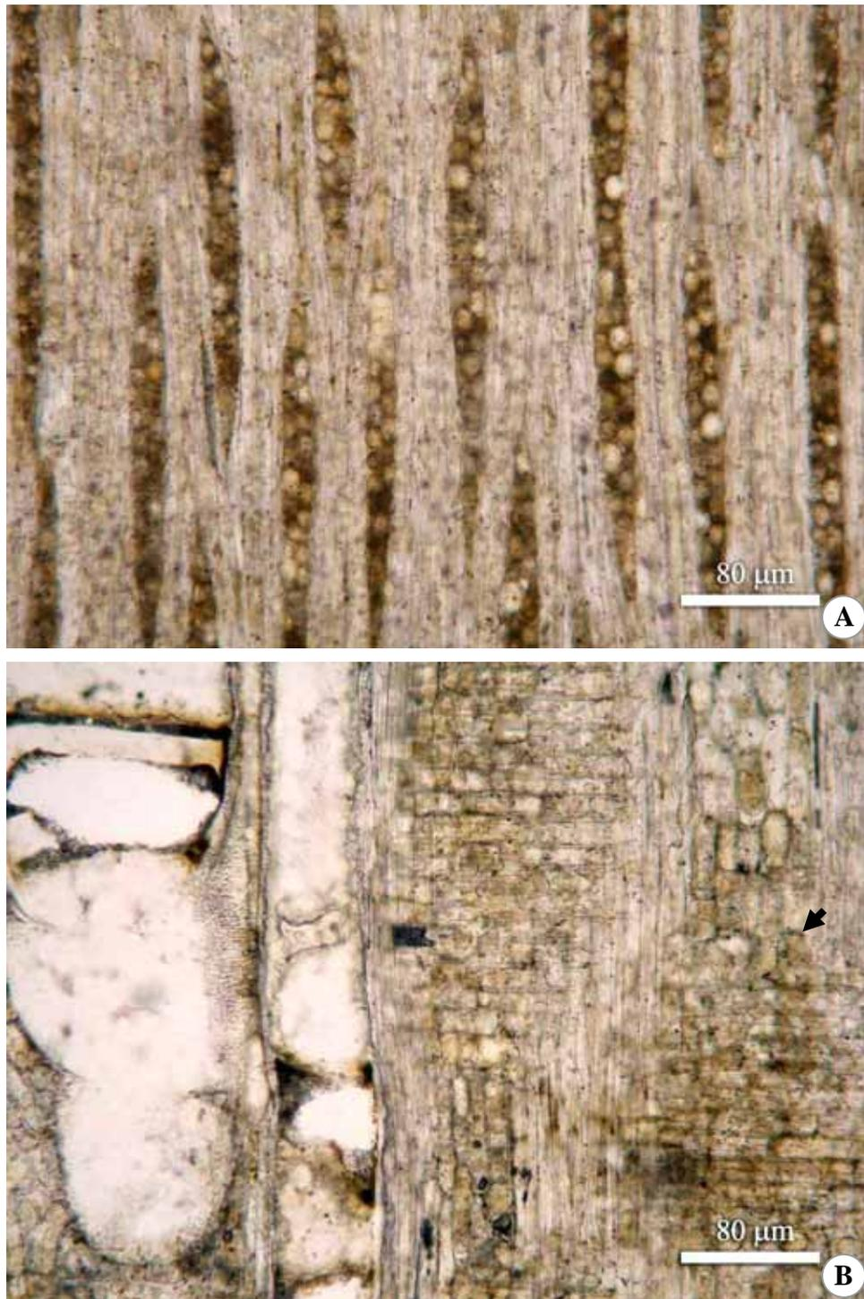
**Figure 4.57** Thin section of fossil wood M1-1. **A.** (Tg) Biseriate and non-storied rays and non-septate fibers. **B.** (R) Body ray cells procumbent with one row of square marginal cells (arrows).
