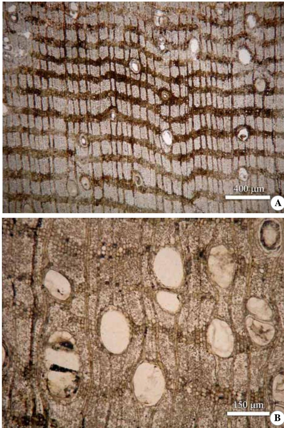
**Figure 4.55** Thin section of fossil wood M1-1. **A.** Solitary vessels are majority. Axial parenchyma bands alternating with fiber bands. Vessels occasionally in radial multiples of 2 - 3.
