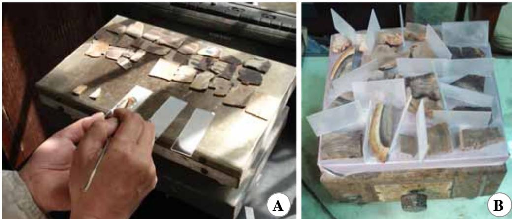
**Figure 3.10** Drying petrified wood specimens and polished slides on a hot plate and using the heat to fix a specimen onto a slide with Abienic Balsam in laboratory of NIGPAS (A) and Department of Geology, CMU (B). The glass slides in the right figure are shorter than those in the left figure.
