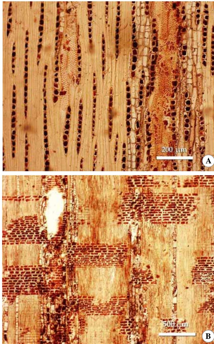
**Figure 4.25** Thin section of modern wood, *Terminalia tomentosa*. **A.** (Tg) Rays exclusively uniseriate and non-storied; alternate intervessel pitting; non-septate fibers. **B.** (R) Homogeneous rays consisting of all procumbent ray cells.
