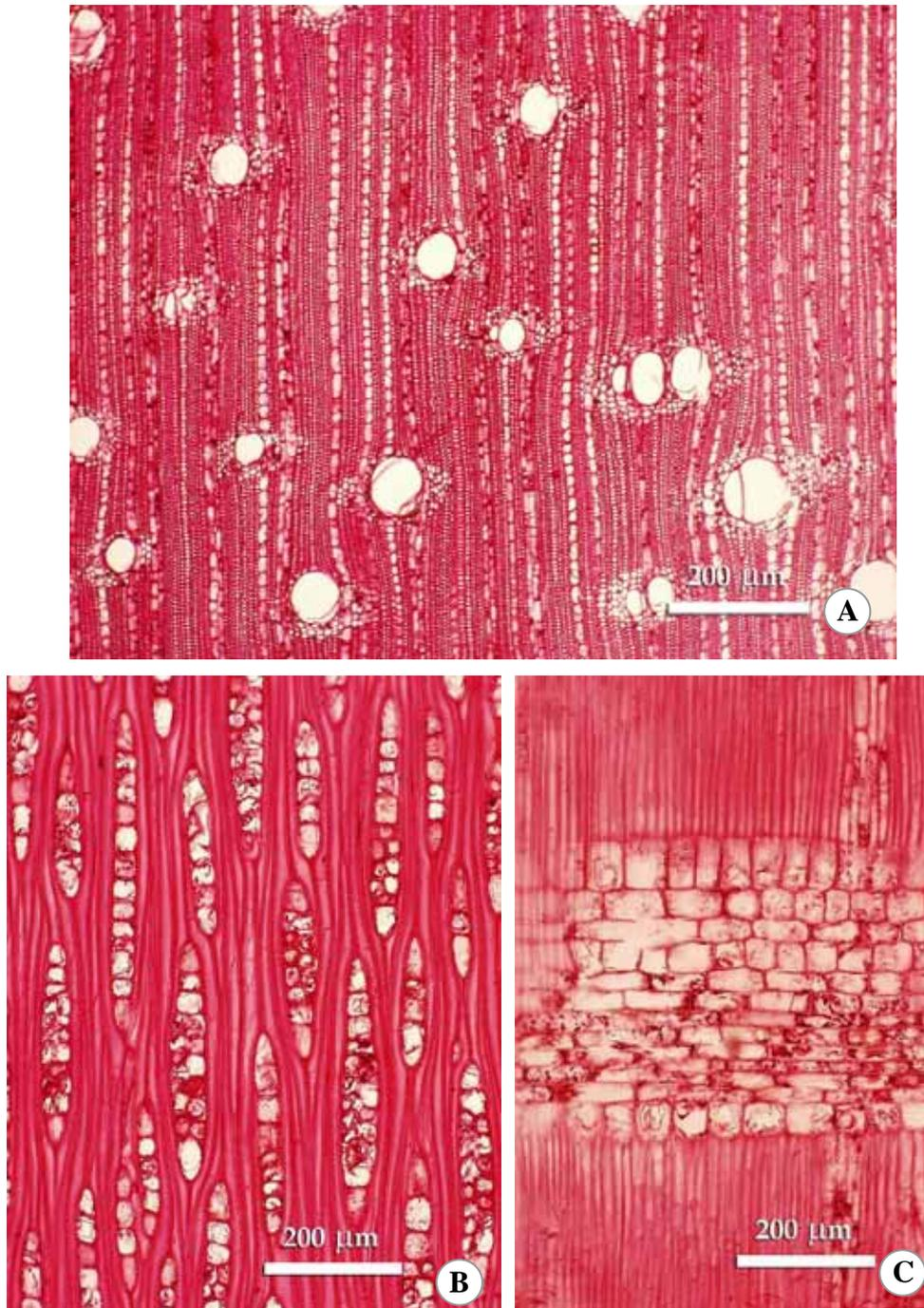
**Figure 4.13** Thin section of *Mangifera caloneura*. **A.** (Tv) Axial parenchyma lozenge-aliform to confluent. **B.** (Tg) Uniseriate (partially 2-seriate) or 1 - 2 seriate rays, non-storied, and non-septate fibers. **C.** Rhomboidal crystals present in ray cells; body ray cells procumbent with a row of upright or square marginal cells.
