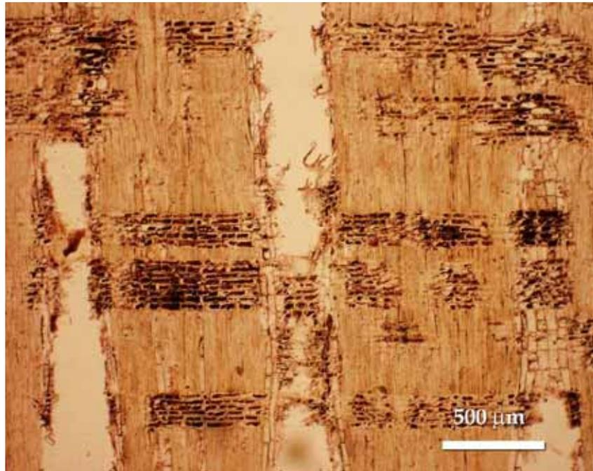
**Figure 4.23** Thin section of modern wood, *Terminalia arjuna*, showing Homogeneous rays consist of all procumbent ray cells.
