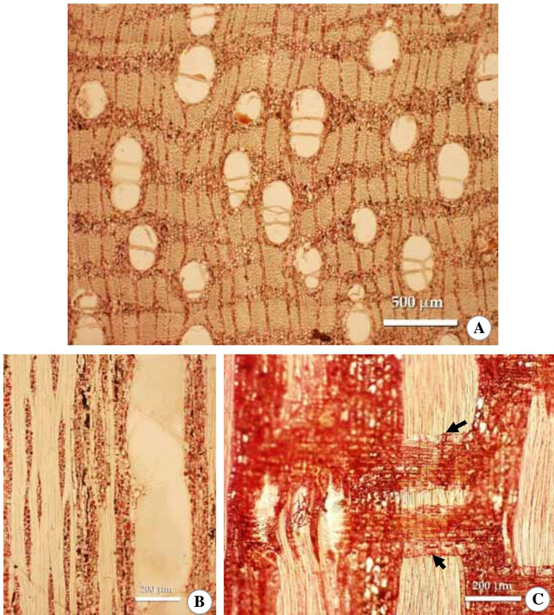
**Figure 4.41** Thin section of modern wood, *Cynometra ramiflora*. **A.** (Tv) Banded parenchyma alternating with fibers bands. Vessels solitary and in radial multiples of 2 - 4. Fibers very thick-walled. **B.** (Tg) Rays (1) 2 (3) seriate and non-seriate. Intervessel pits alternate. **C.** (R) Body ray cells procumbent with one row of upright and/or square marginal cells (arrow). Vessel-ray pits with distinct borders, similar to intervessel pits in size and shape throughout the ray cells.
