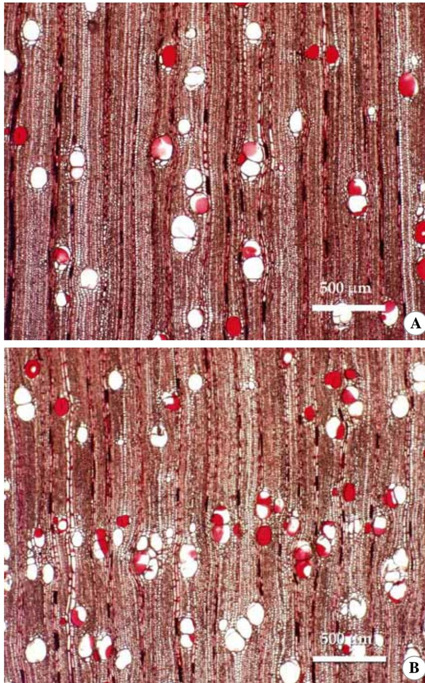
**Figure 4.69** Thin section of *Azadirachta excelsa*. **A.** (Tv) Solitary vessels common, some in radial multiples and clusters. **B.** (Tv) Irregular band of axial parenchyma and vessel clusters.
