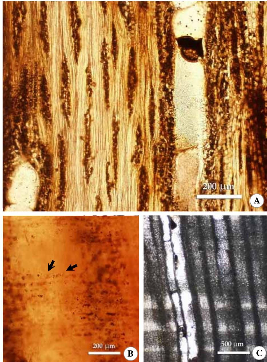
**Figure B16** Thin section of slide no. NRRU-60 (A and B). **A.** (Tg) Non-storied and 1 - 3 seriate rays, non-septate fibers, alternate intervessel pits, and deposits appearing to collect at the ends of vessel elements. **B.** (R) Body ray cells procumbent with one row of square/upright marginal cells (arrow). **C.** (R) Thin section of slide no. M8 showing vessels elements and pattern of rays.
