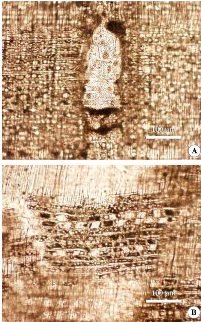
**Figure 4.8** Thin section of slide G5 in radial section. **A.** Vessel-ray pits with distinct borders; similar to intervessel pits in size and shape throughout the ray cell. **B.** Rhomboidal crystals in ray cells.
