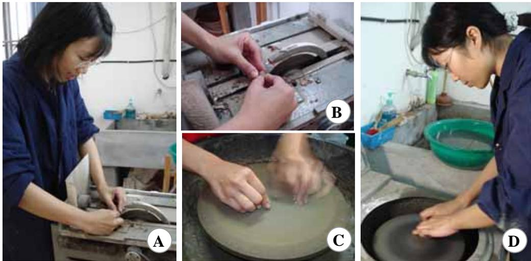
**Figure 3.9** Cutting (A& B) and polishing (C & D) petrified wood specimens.
