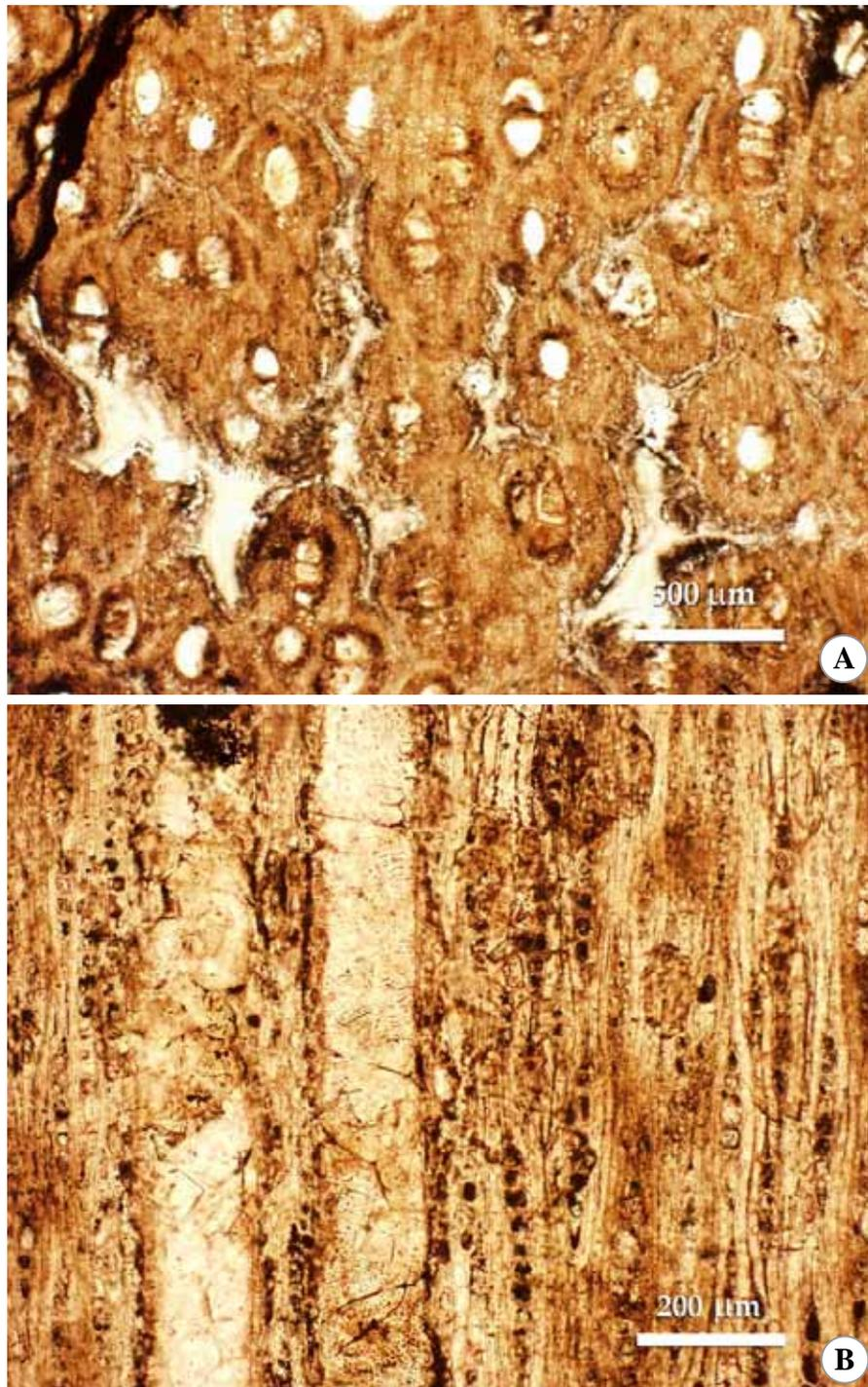
**Figure 4.20** Thin section of slide no. A4-1. **A.** (Tv.) Vessels solitary and in radial multiples of 2 - 4 and axial parenchyma vasicentric to lozenge-aliform. **B.** (Tg.) Mostly uniseriate rays and a few 1 (with partially 2) seriate rays. Intervessel pits can be seen on the vessel walls.
