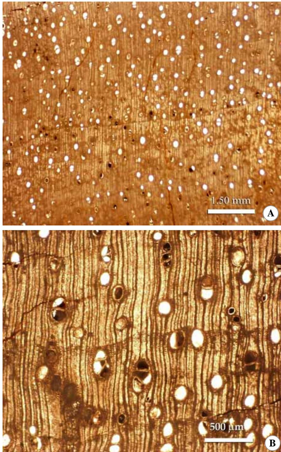
**Figure 4.10** Thin section of N7 - 3 (Tv). **A.** Diffuse-porous distribution of vessels.
