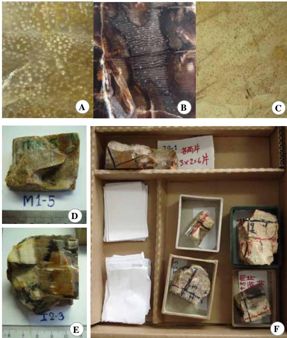
**Figure 3.7** A. - C. show the well preserved areas of the specimens in transverse section. D. & E. show petrified wood pieces, about 4x4x4 cm or 5x5x5 cm, that were selected and cut from the field. F. The specimens were marked for cutting into three sections and separated in each box.
