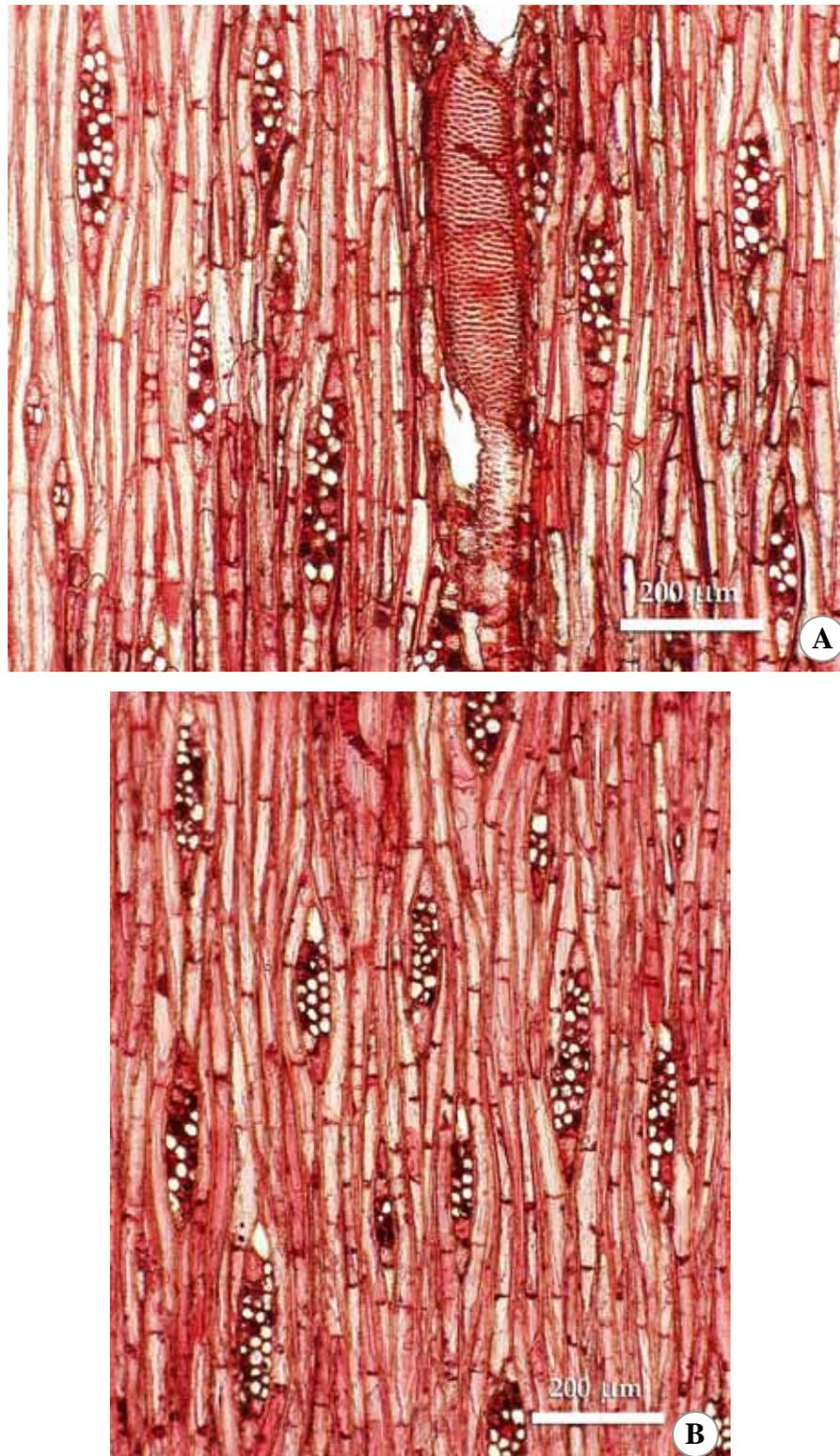
**Figure 4.18** Thin section of *Canarium venosum* in tangential section. **A.** Alternate intervessel pitting. **A.** and **B.** Non-storied, 1 - 3 seriate rays, and septate fibers.
