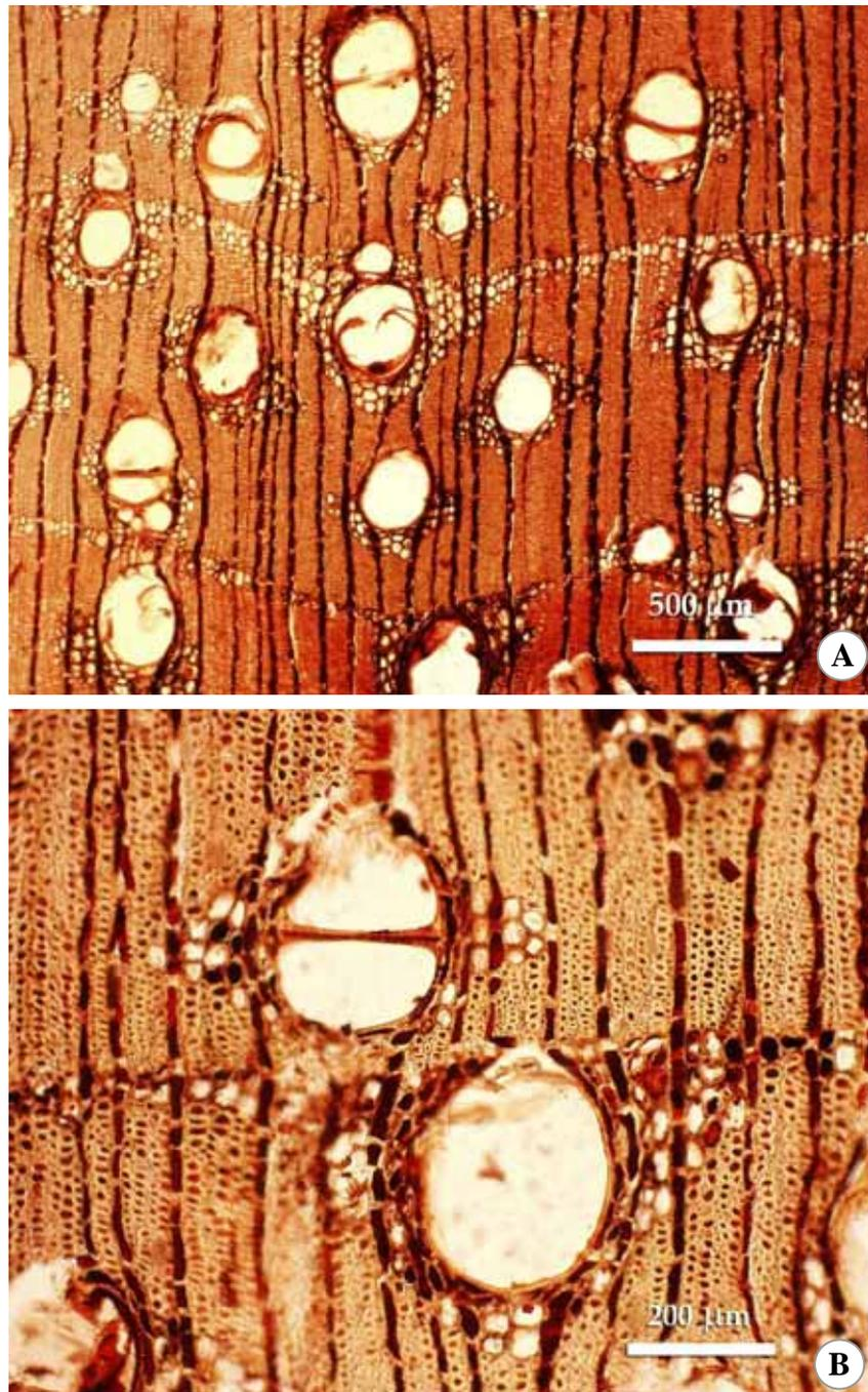
**Figure 4.24** Thin section of modern wood, *Terminalia tomentosa* (slide no.FRI876), in transverse section. **A.** and **B.** Vessels solitary or in radial multiples of 2; axial parenchyma aliform and in marginal or seemingly marginal bands. **B.** Fibers thin-to thick-walled.
