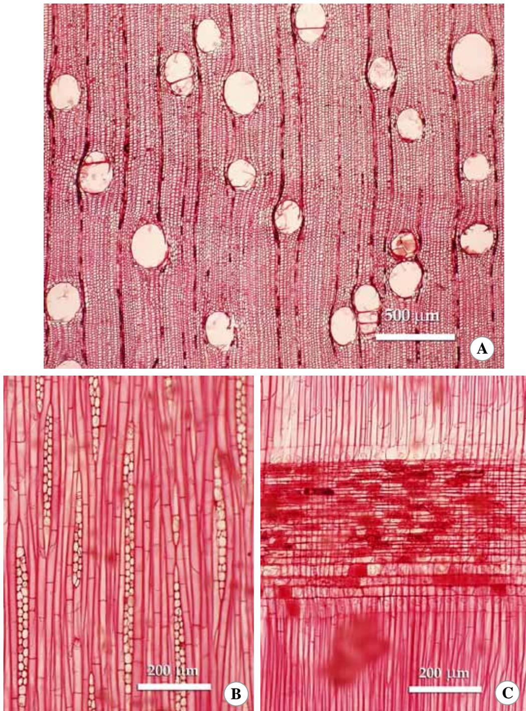
**Figure 4.5** Thin section of *Dracontromelon* sp. **A.** (Tv) Vessels solitary and in radial multiples of 2 - 3. **B.** (Tg) Exclusively biseriate and non-storied rays and septate fibers. **C.** (R) Rhomboidal crystals in hexagonal shape present in ray cells; body ray cells procumbent with 1 - 3 rows of upright and/or square marginal ray cells.
