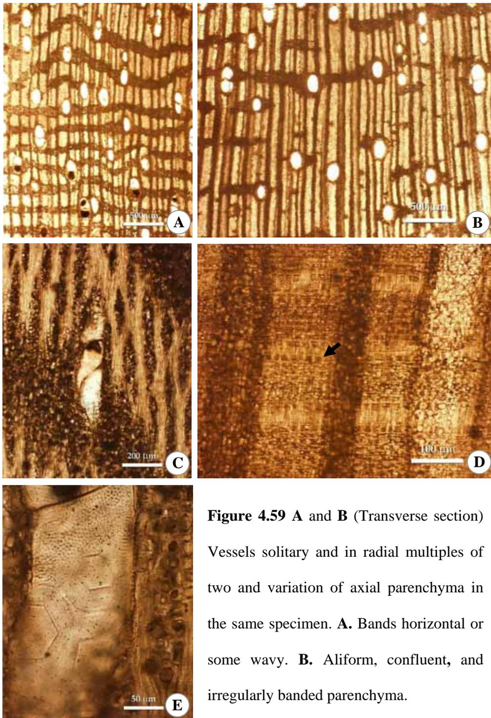
**C.** (Tg) Irregularly storied or occasionally non-storied, 2 - 3 seriate rays; non-septate fibers. **D.** (R) Body ray cells procumbent with 1 row of square/upright marginal cells (arrow). **E.** (Tg) Alternate intervessel pits.
