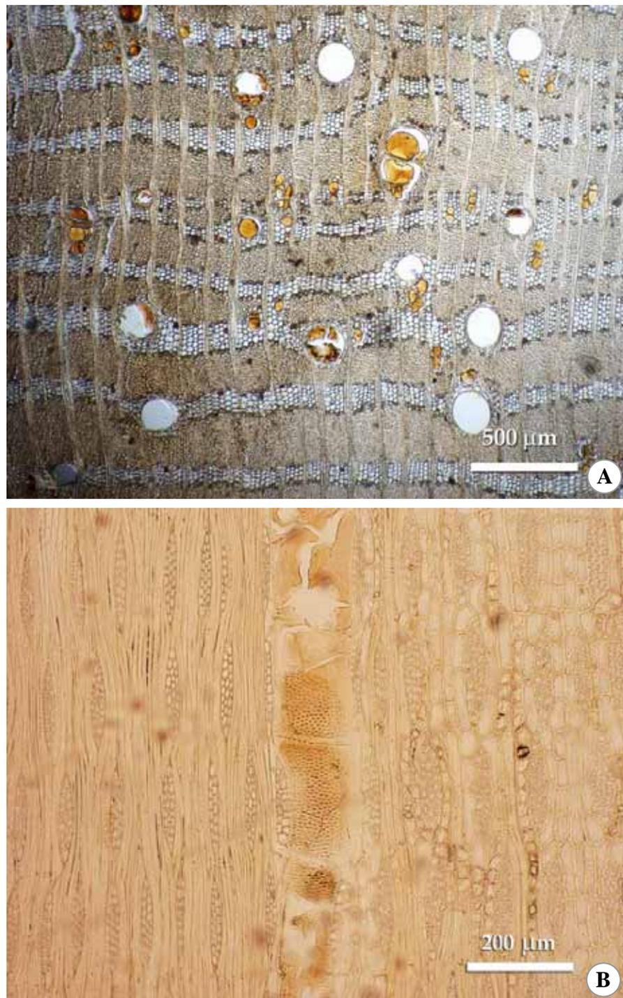
**Figure 4.50** Thin sections of modern wood, *Millettia leucantha*. **A.** (Tv) (slide no. FRI636) Banded parenchyma alternate with fiber bands. **B.** (Tg) (slide no. FRI610) 1 - 3 seriate rays in storied arrangement. Non-septate fibers, alternate intervessel pits, and prismatic crystals in chambered axial parenchyma cells.
