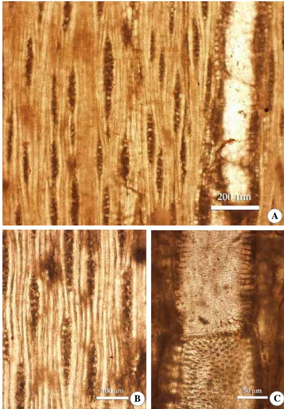
**Figure B2** Thin section of fossil wood M7-2. **A.** and **B.** (Tg) Non-storied, 1 - 2 seriate rays and non-septate fibers. **C.** (Tg) Alternate intervessel pitting can be observed from vessels wall.
