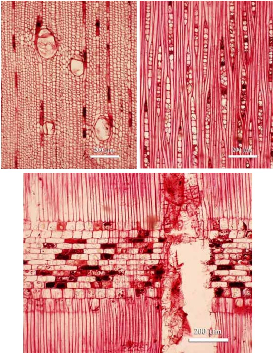
**Figure 4.9** Thin section of *Mangifera camptosperma*. **A.** (Tv) Solitary vessels and radial multiples of 2; axial parenchyma vasicentric. **B.** (Tg) Rays 1 (or partially 2) seriate, non-storied; and non-septate fibers. **C.** (R) Rays consisting of procumbent body ray cells and square or upright marginal cells. Rhomboidal crystals in ray cells.
