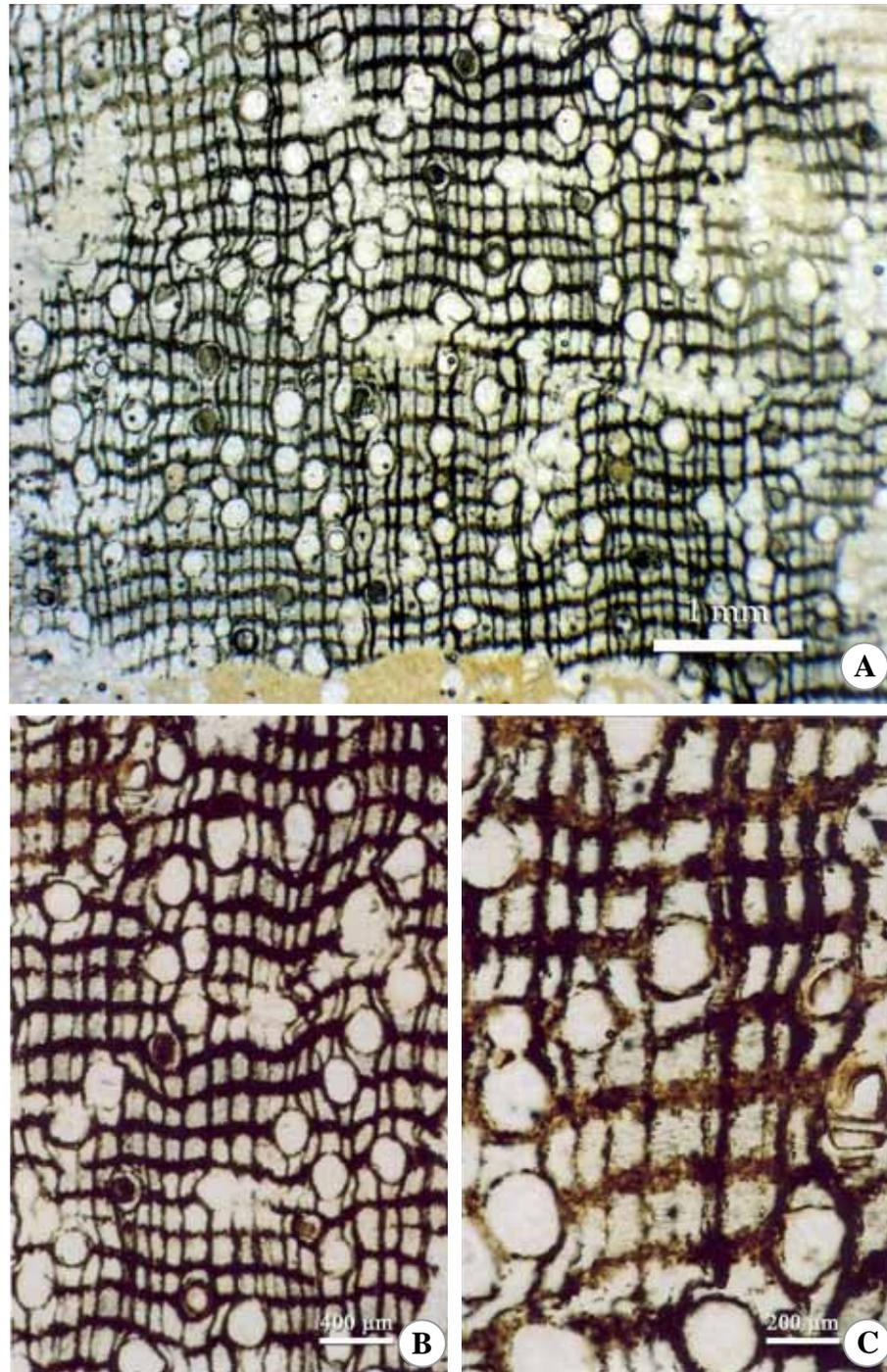
**Figure 4.30** Thin section of fossil wood L7 in transverse section. **A.** and **B.** Axial parenchyma in continuous narrow bands in similar width as the rays, but mostly parenchyma rather thicker, appearing reticulate. **C.** Fibers very thick-walled.
