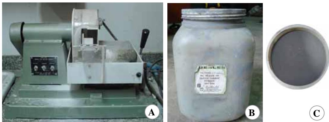
**Figure 3.5 A.** Ingram thin section grinder. **B. & C.** Silicon carbide abrasive powder.
