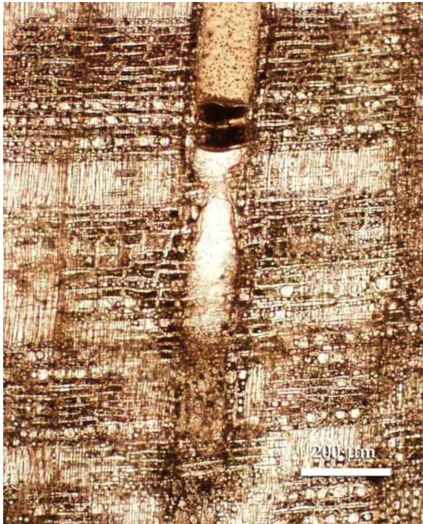
**Figure 4.7** Thin section of slide G5 in radial section. Heterogeneous rays. Some rays consisting of all procumbent cells and some with procumbent and square cells mixed throughout the ray.
