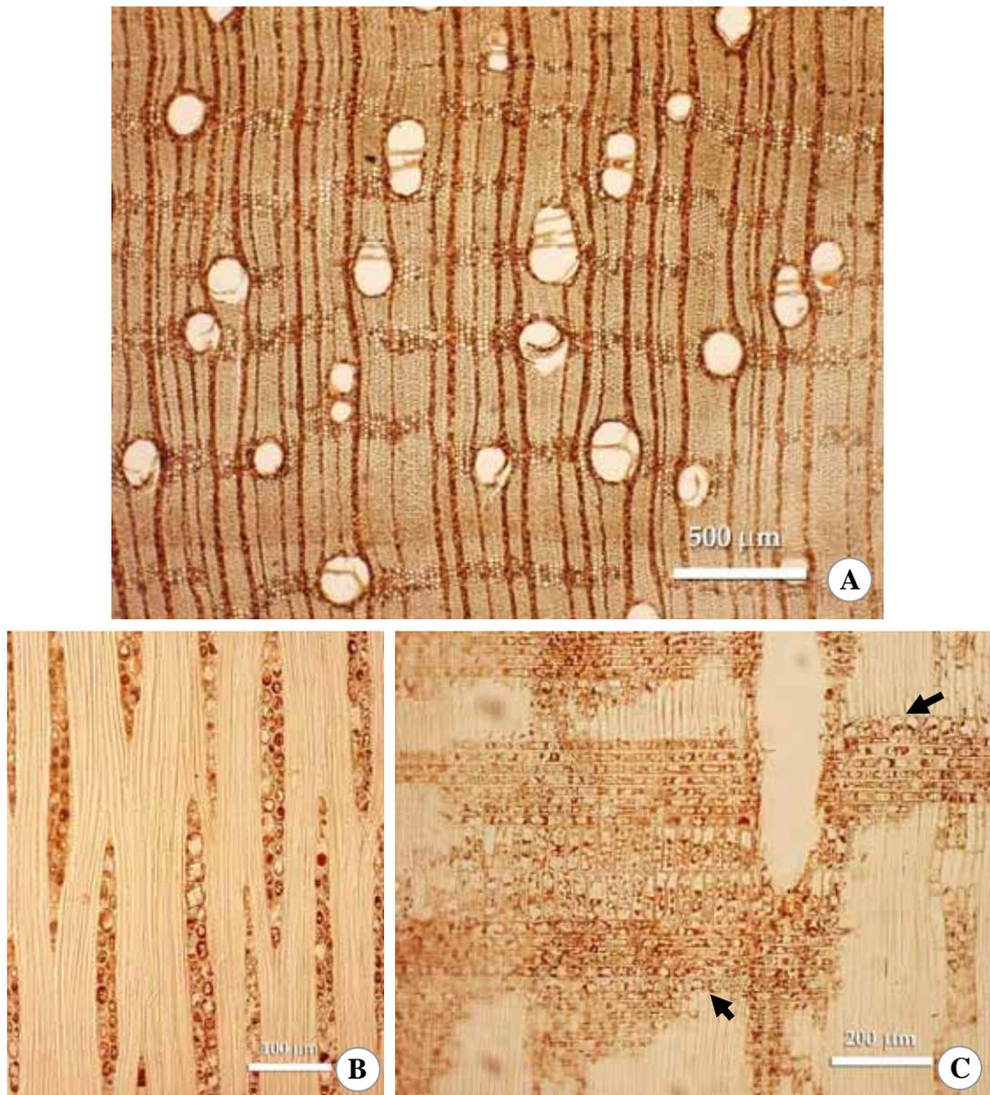
**Figure 4.42** Thin section of modern wood, *Cynometra polyandra* **A.** (Tv) Banded parenchyma alternating with fibers bands. Vessels solitary and in radial multiples of 2 - 4. Fibers very thick-walled. **B.** (Tg) Rays (1) 2 (3) seriate and non-storied. **C.** (R) Body ray cells procumbent with one row of upright and/or square marginal cells (arrow).
