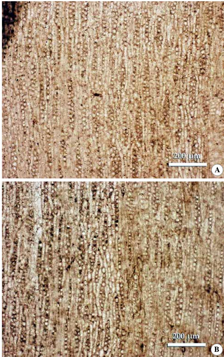
**Figure 4.48** Thin section of fossil wood C4, tangential section. **A.** Storied rays
