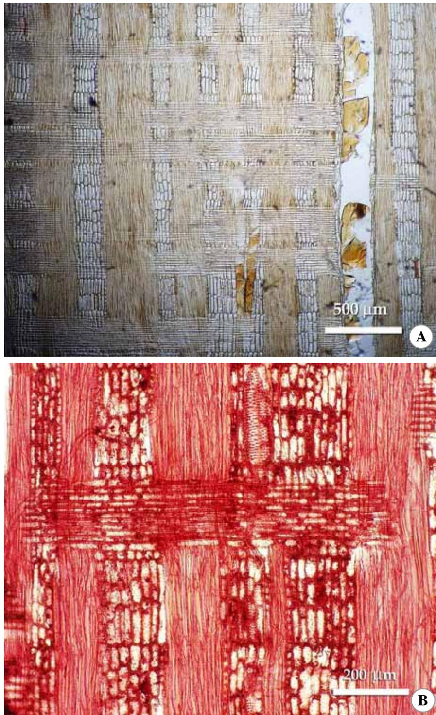
**Figure 4.51** Thin sections of modern wood, *Millettia leucantha*. **A.** (R) (slide no. FRI636) Homogeneous ray tissues. **B.** Homocellular ray cells are all procumbent.
