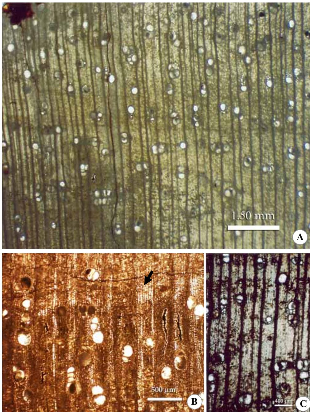
**Figure 4.66** Thin section of A4-2. Transverse section. **A.** and **C.** Solitary and clusters of vessels are common. **B.** Irregular band of 10 - 16 cells axial parenchyma cells (arrow) and some radial multiples of 2 - 4 vessels.
