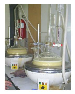
Figure 2.1 A Cleveneaur's distillation apparatus used in the extraction process.
