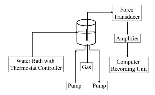
Figure 2.2 Schematic representation of the set up used for tension measurements.
