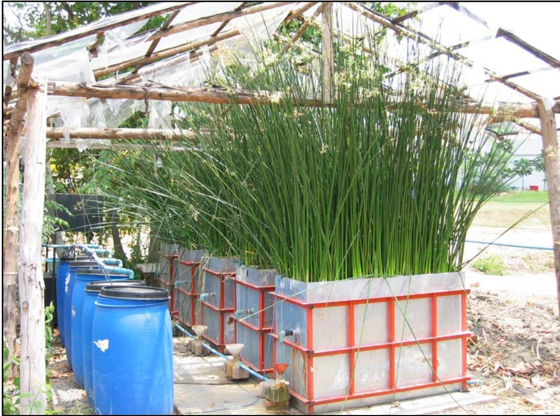
**Figure 3.3** The five FWS constructed wetland units and head tanks.
