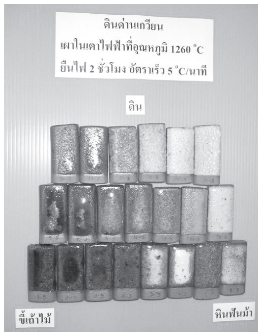
Figure 6. Dan Kwian biscuits coated with Celadon glazes and fired in an electric kiln to the maximum temperature of 1,260°C with a heating rate of 5°C/min and a soaking time of 2 h. No glaze peeled out from its biscuit
