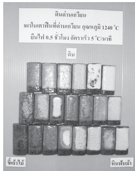
Figure 7. Dan Kwian biscuits coated with Celadon glazes and fired in Dan Kwian kiln to the maximum temperature of 1,240°C with a heating rate of 5°C/min and a soaking time of 0.5 h. No glaze peeled out from its biscuit
