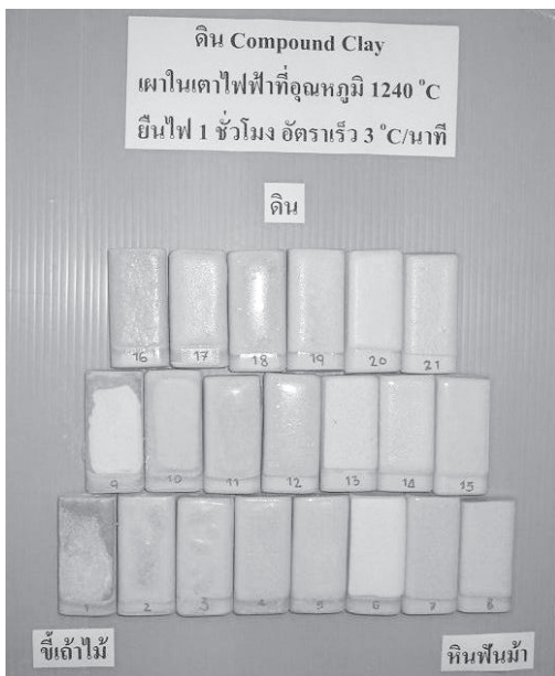
Figure 8. Compound clay biscuits coated with Celadon glazes and fired in an electric kiln to the maximum temperature of 1,240°C with a heating rate of 3°C/min and a soaking of time 1 h. Glaze formulae #1 and #9 peeled out from their biscuits
