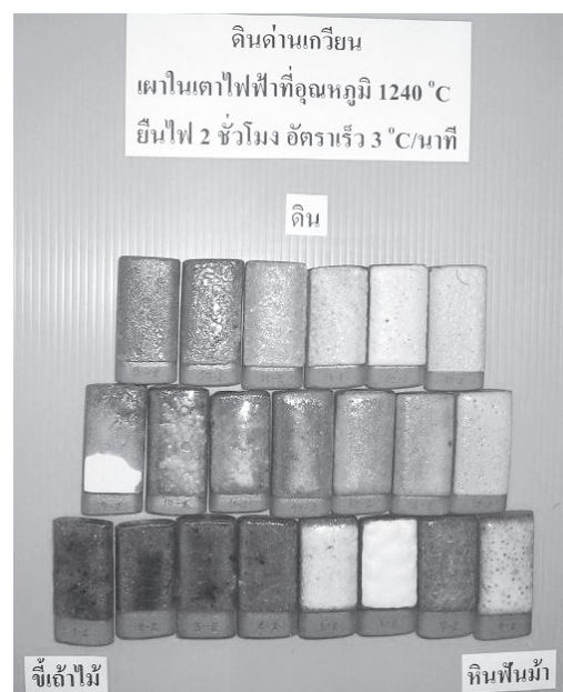
Figure 5. Dan Kwian biscuits coated with Celadon glazes and fired in an electric kiln to maximum temperature of 1,240°C with a heating rate of 3°C/min and a soaking time of 2 h. Glaze formula #9 peeled out from its biscuit
