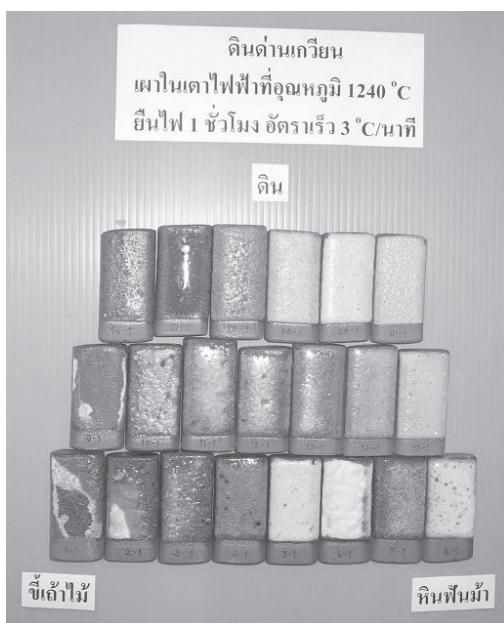
Figure 4. Dan Kwian biscuits coated with Celadon glazes and fired in an electric kiln to the maximum temperature of 1,240°C with a heating rate of 3°C/min and a soaking time of 1 h. Glaze formulae #1, #2, and #9 peeled out from their biscuits
